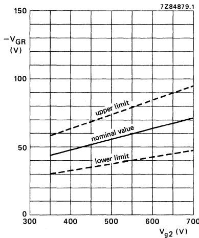
Limits of grid 1 cut-off voltage as a function of grid 2 voltage.
