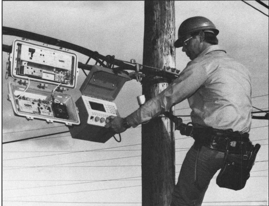
Figure 1. The light and compact 2722 Sweep Receiver with its high visibility display brings a new level of efficiency and capability to in-service CATV system testing.
