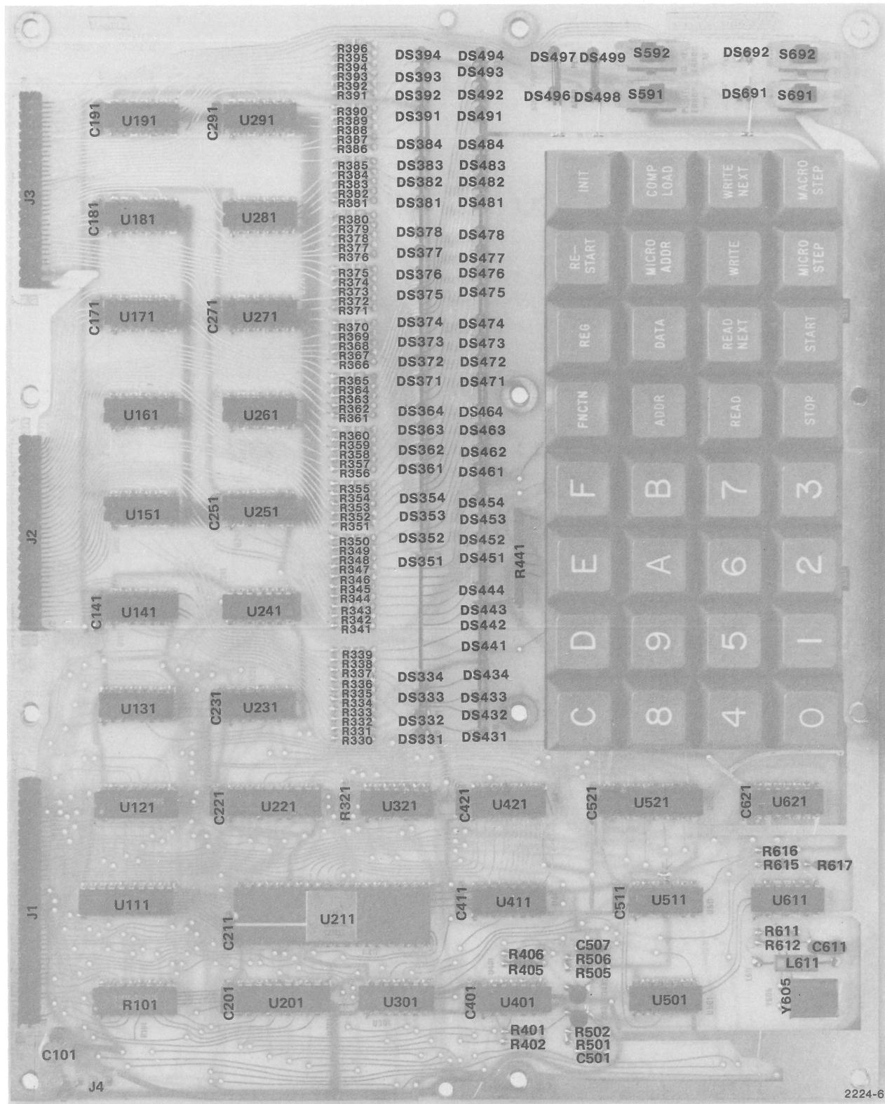
Test Fixture Controller Component Locations (670-5728-00).
