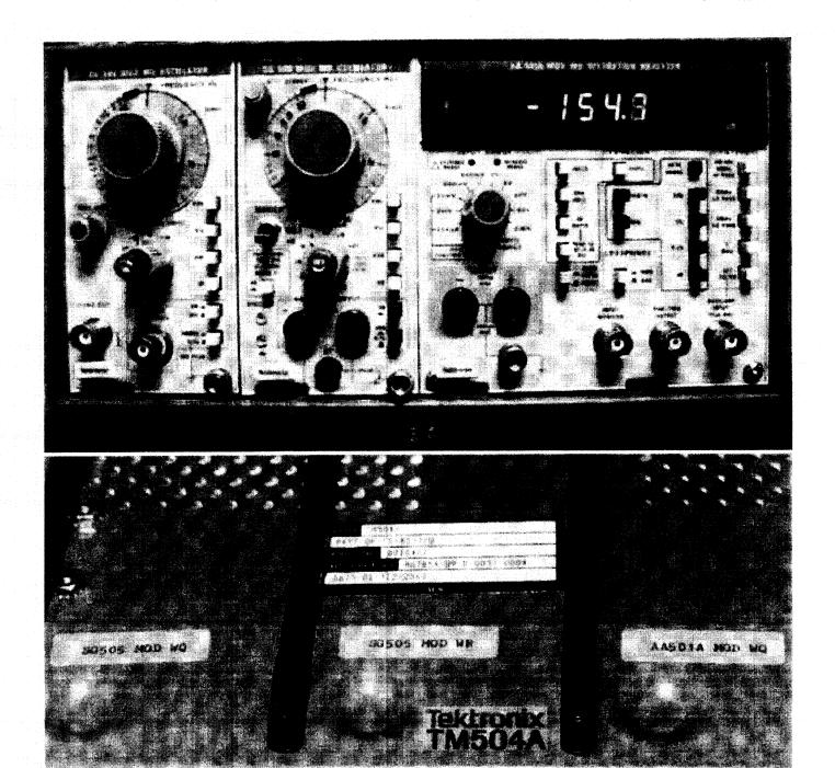
Positioning of the plug-ins in the TM504A case for cross-talk capability. See notes about the differences in the standard TM504 and TM504A backplane.
