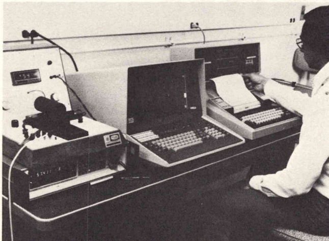
Fig. 1. The Tektronix 4051 Graphic System is the controller in the automated system which analyzes pelleted samples for uranium. A fluorometer modified to include a digital voltmeter (left), and a printer/storage terminal (right) complete the system.
