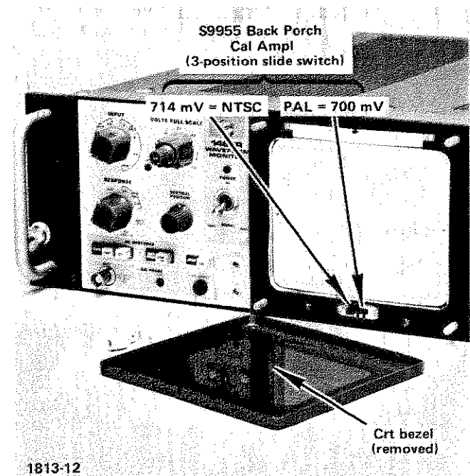
Fig. 2-6. Location of BACK PORCH CAL AMPL S9955. (Same location in cabinet models.)
