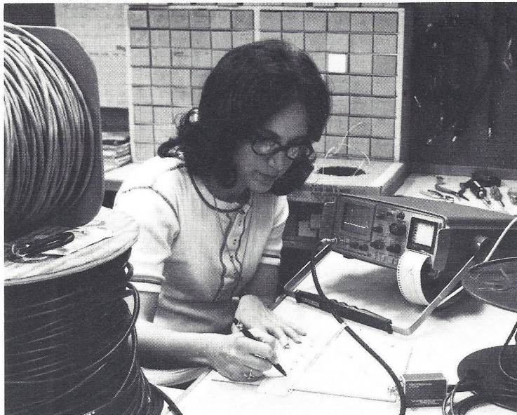
LOUISE GRAY (Spectrum Analyzers) checks output of Tek's 1503 TDR Cable Tester. This model has the optional chart recorder.
