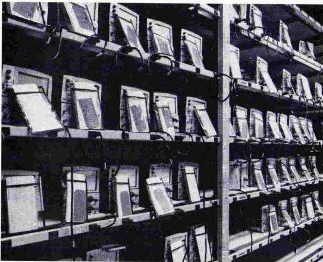
Fig 5. Partial view of cycle rack where T900s undergo 7-day burn-in cycle at elevated temperatures.
