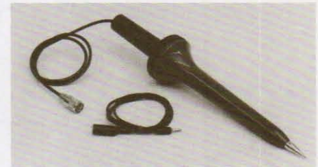
Model 6103C Voltage Divider Probe: Permits voltage measurement to 30kV and has a 1000:1 division ratio. Accuracy is ±5% of reading. Its 4.5 \times 10^{11} \Omega input resistance permits use with Keithley electrometers and other high impedance multimeters. Connector is a UHF male plug. Requires the 6012 Coaxial to Triaxial Adapter when used with Models 602, 614, 616 and 619. Lead length is 0.8m (30 in.).
