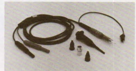
Model 1682A RF Probe (DMMs) AC to DC Transfer Accuracy: \pm 1 dB from 100kHz to 250MHz at 1V, peak responding, calibrated in rms of a sine wave, compatible with instruments with 10M \Omega input resistance. Voltage Range: 0.25V to 15V rms. Maximum Allowable Input: 42V AC peak, 200V (DC + AC peak).
