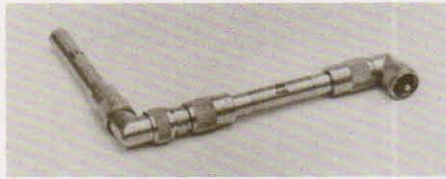
Model 2503 Static Detector Probe: Designed to detect voltage due to charge on relatively small surface areas. Solid coaxial 13mm (1/2 in.) diameter tube used with 89mm (3 1/2 in.) head, 89mm (3 1/2 in.) coupler, 25mm (1 in.) adapter and two 90° angle adapters which may be placed at various junctions along the tube. It gives a 10,000:1 ±10% division ratio when used with Model 610C and held 6mm (1/4 in.) away from a charged plane of at least 13mm (1/2 in.) diameter. Output is a UHF male plug.
