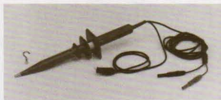
Model 1600A High Voltage Probe (DMMs) Maximum Input: 40kV DC or peak AC to 300Hz. Input Resistance: 1000M \Omega . Division Ratio: 1000:1 (into 10M \Omega ). Ratio Accuracy (into 10M \Omega DMM): \pm 2.5\% from 1kV to 40kV DC; -3dB at 300Hz AC. Operating Temperature: 0° to 50°C.
