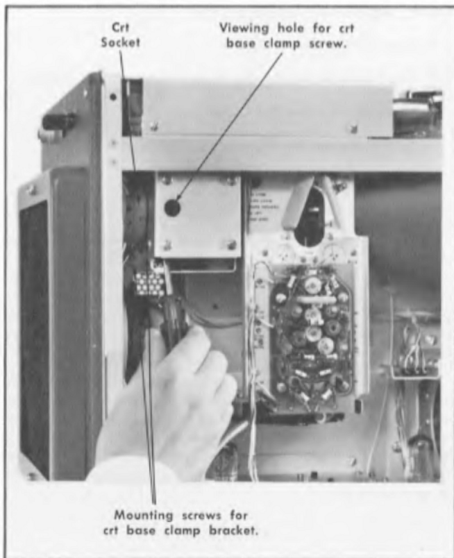
Fig. 4-3. Loosening the crt base clamp.
