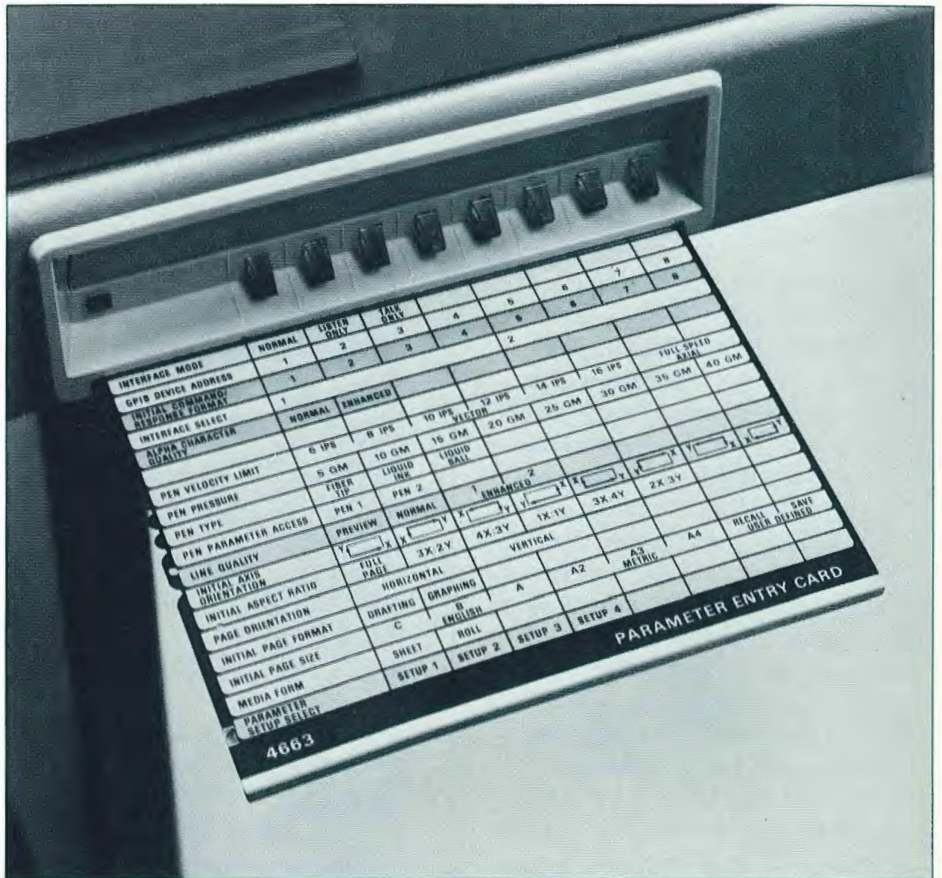
Fig. 1. Parameter entry device simplifies plotter set up and servicing.
