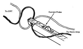
Fig. 5-29. Proper connection of current probe to horizontal deflection leads for high-speed timing calibration.
