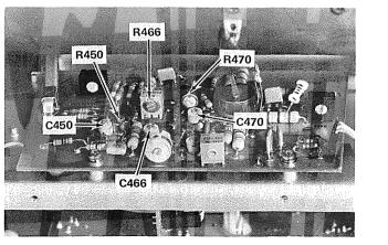
Fig. 5-16. Location of vertical output high-frequency adjustments.
