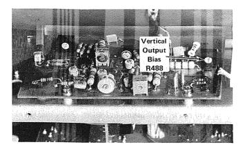
Fig. 5-5. Location of Vertical Output Bias adjustment.
