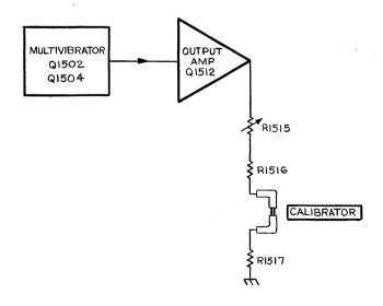
Fig. 3-10. Detailed block diagram of the Calibrator.
