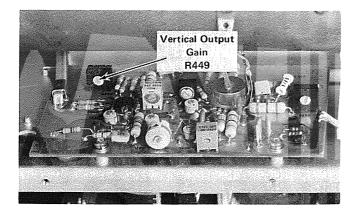
Fig. 5-13. Location of Vertical Output Gain adjustment.
