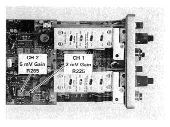
Fig. 5-14. Location of Gain adjustment for Channel 2.
