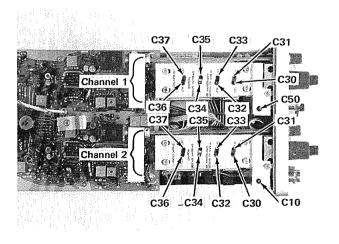
Fig. 5-19. Location of VOLTS/DIV Compensation adjustments.
