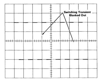
Fig. 5-1. Typical CRT display when checking chopped blanking.
