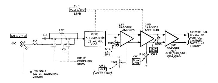
Fig. 3-2. Detailed block diagram of the Channel 1 Vertical Preamplifier circuit.
