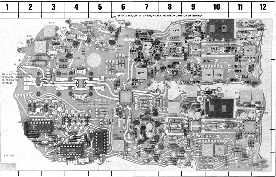
Fig. 7-5. P/0 A3 Vertical Preamp circuit board.
