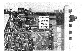
Fig. 5-6. Location of Vertical Shield Voltage adjustment.
