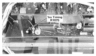
Fig. 5-28. Location of 1 nanosecond timing adjustment.
