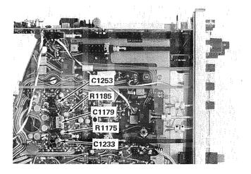
Fig. 5-27. Location of high-speed timing adjustments (except R1075).
