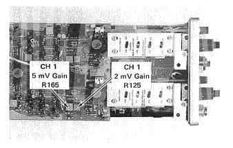
Fig. 5-12. Location of Gain adjustments for Channel 1.
