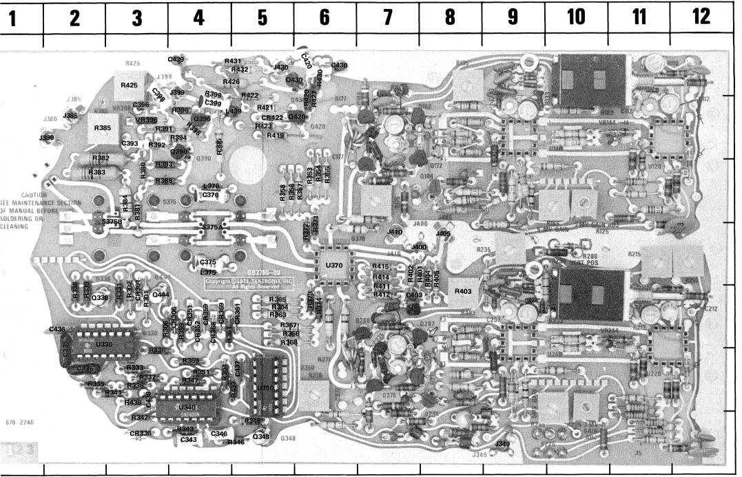
Fig. 7-10. P/0 A3 Vertical Preamp circuit board.
