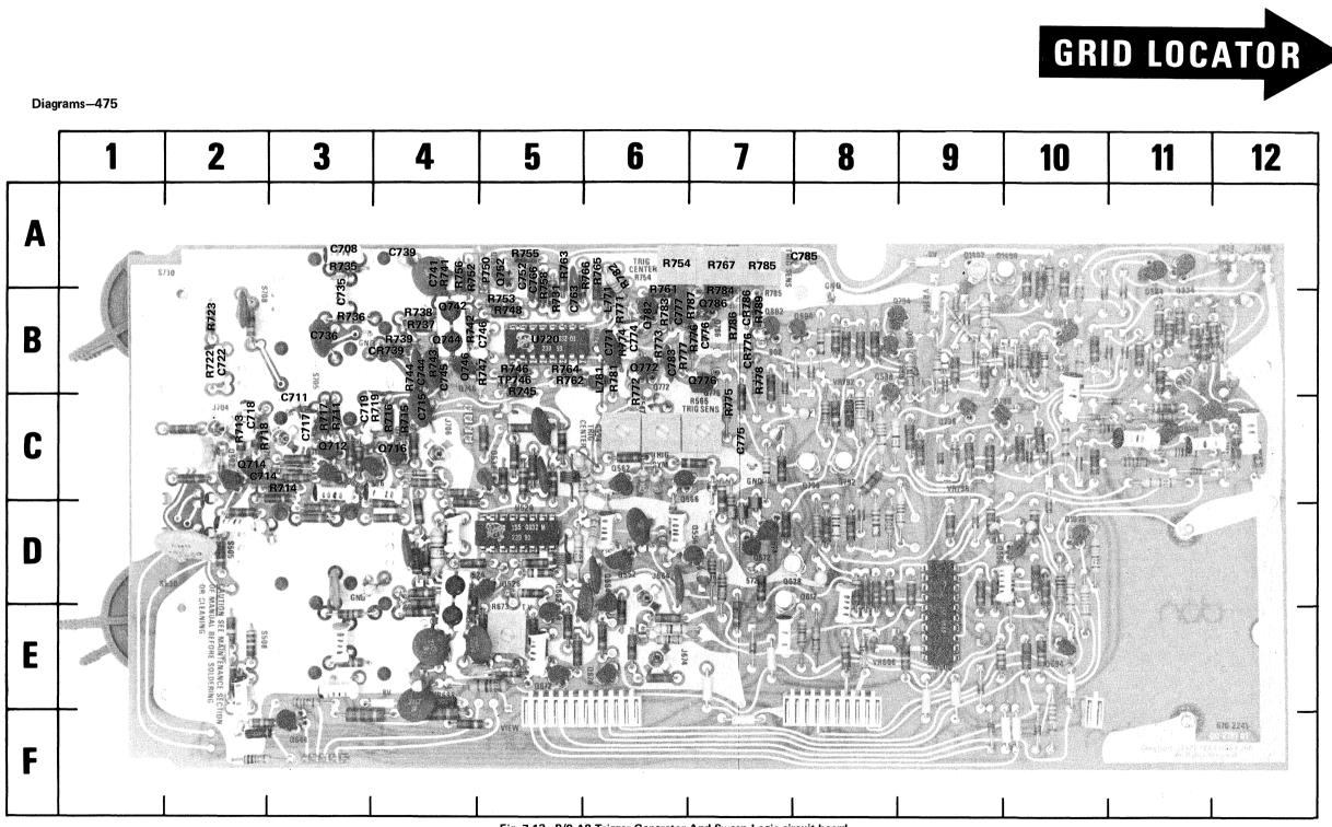
Fig. 7-13. P/0 A8 Trigger Generator And Sweep Logic circuit board.
