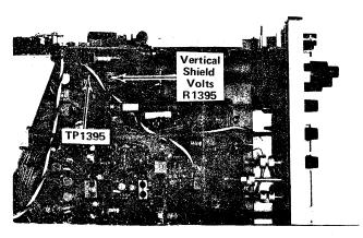
Fig. 5-6. Location of Vertical Shield Voltage adjustment and TP1395.
