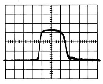
Fig. 5-30. Typical CRT display with high-speed timing adjustments preset.
