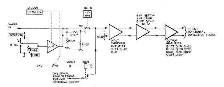
Fig. 3-7. Detailed block diagram of the Horizontal Amplifier.
