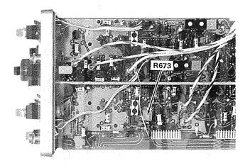
Fig. 5-22. Location of Trigger View Centering adjustment.
