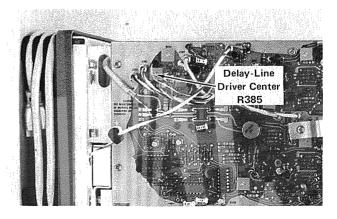
Fig. 5-7. Location of Delay-Line Driver Centering adjustment.
