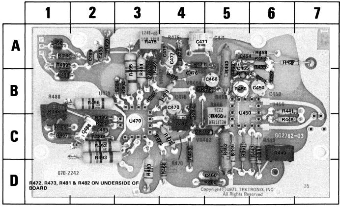
Fig. 7-11. A5 Vertical Output circuit board.
