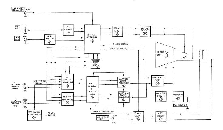
Fig. 3-1. Basic block diagram of the 475.
