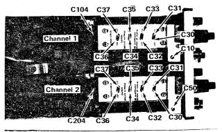
Fig. 5-19. Location of VOLTS/DIV Compensation adjustments.
