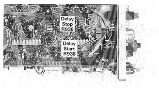
Fig. 5-23. Location of Delay Start and Delay Stop adjustments.
