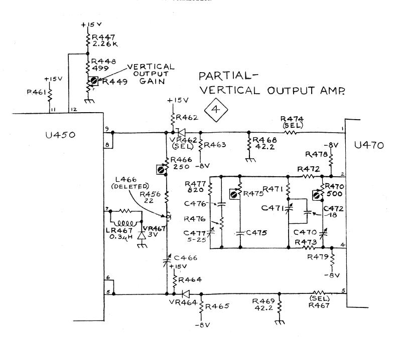
Note: Original schematic was in error, R466 always connected to U450 pins 8 and 9, and C466 always connected to pins 5 and 6 with L466 located between R466 and C466. (This mod removes L466)
