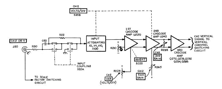
Fig. 3-3. Detailed block diagram of the Channel 2 Vertical Preamplifier circuit.
