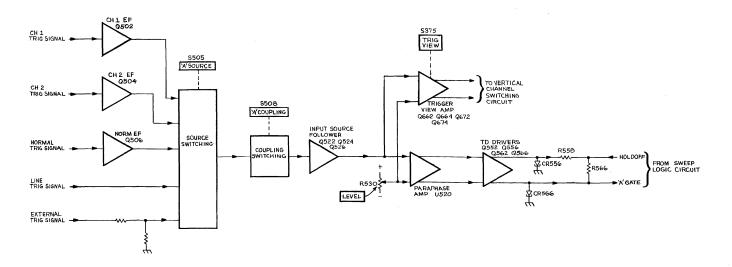
Fig. 3-5. Detailed block diagram of the A Trigger Generator.
