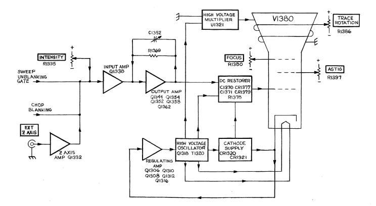
Fig. 3-9. Detailed block diagram of the CRT Circuit.
