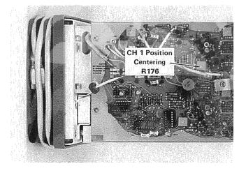
Fig. 5-9. Location of CH 1 Position Centering adjustment.
