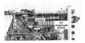
Fig. 5-32. Location of Q1504 and Calibrator amplitude adjustment.
