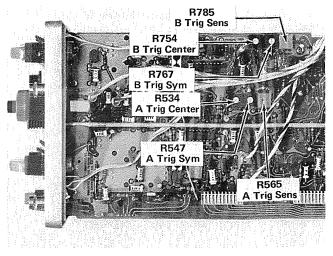
Fig. 5-20. Location of Trigger Sensitivity, Symmetry, and Centering adjustments.
