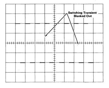
Fig 5-15. Typical CRT display when checking chopped blanking.
