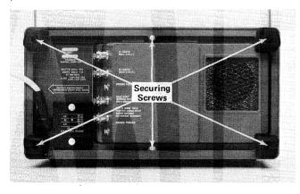
Fig. 4-1. Removing wrap-around cabinet.
