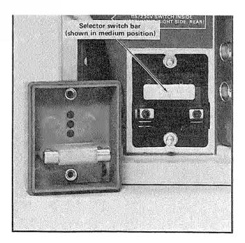
Fig. 2-1. Power supply regulating range selector.
