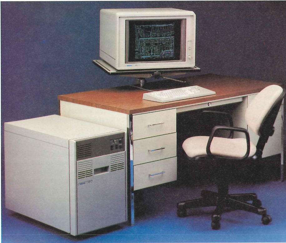
The 4115B is available in two packages: a pedestal configuration shown on the front cover of TEKniques , and the modular configuration shown above which separates the display, keyboard and processing components.
