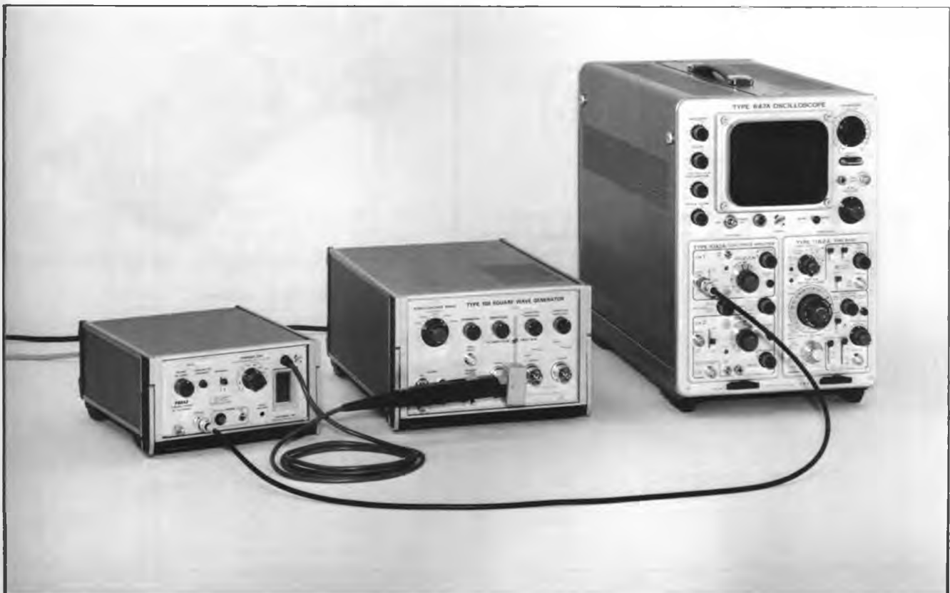
Fig. 2-3. P6042 Current Probe connected to Type 106 Square-Wave Generator output.
