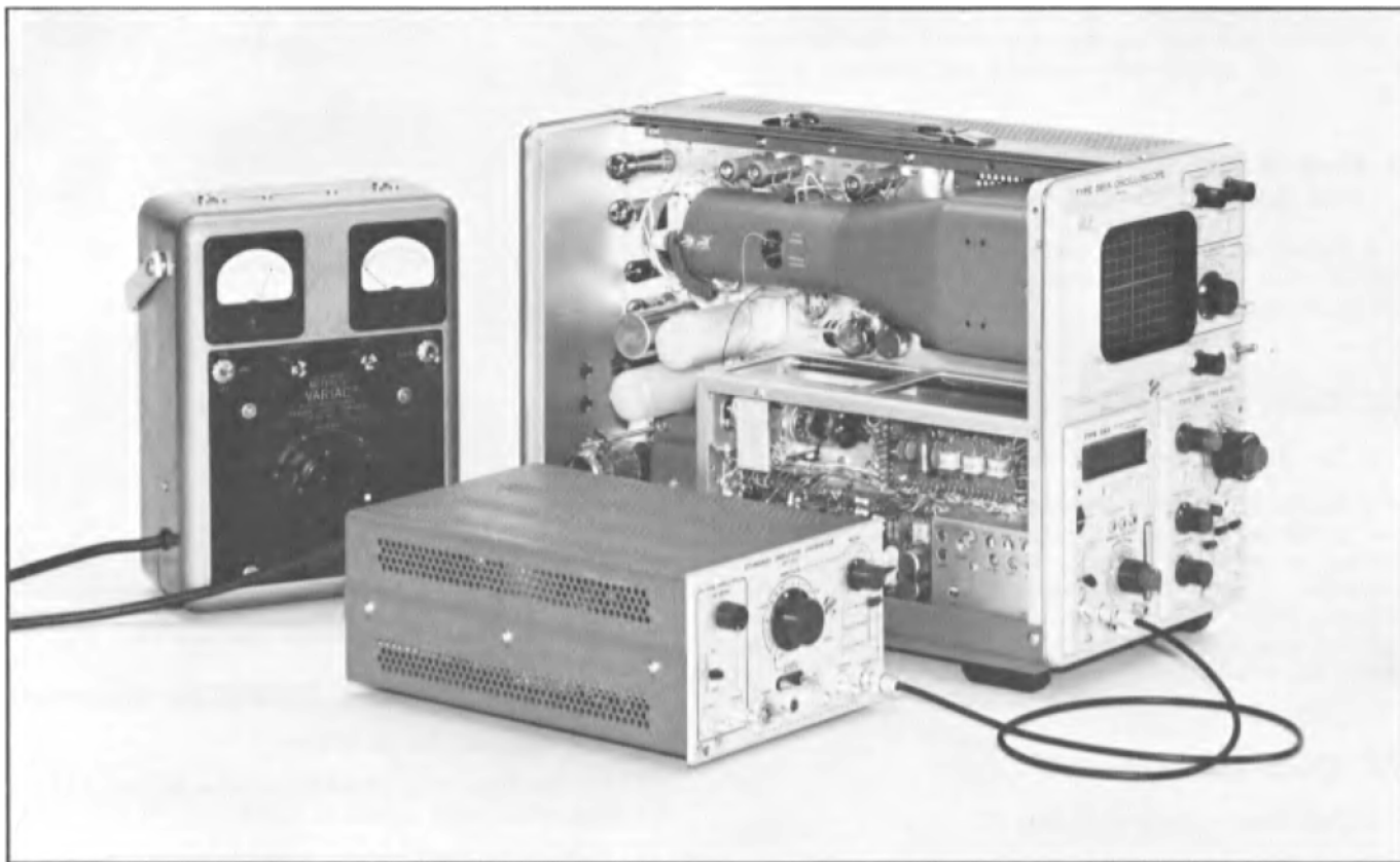
Fig. 6-7. Test setup for adjusting Vertical Amplifier gain.
