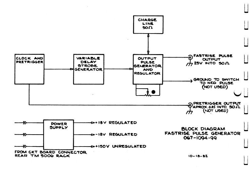
Figure 7-1: Pulse Generator Block Diagram
