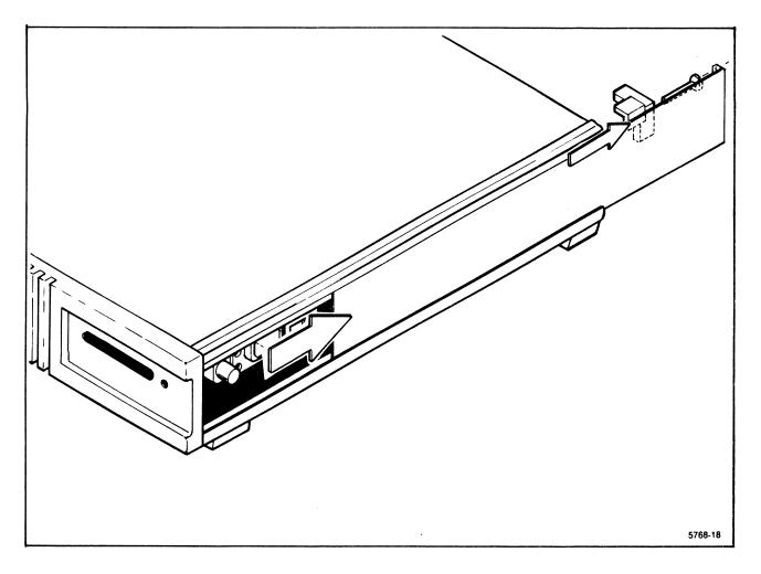
Figure B-2. Exposing the 91HS8 power supply.
