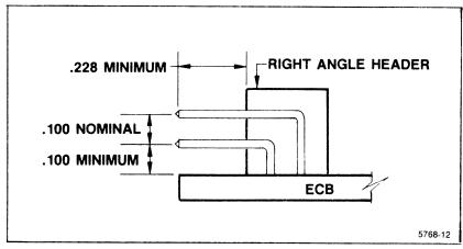
Figure 2. Minimal right-angle square pin spacing for 91HS8 probelets.
