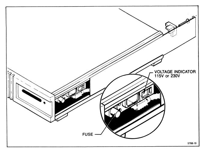
Figure B-3. Selecting a different voltage range.
