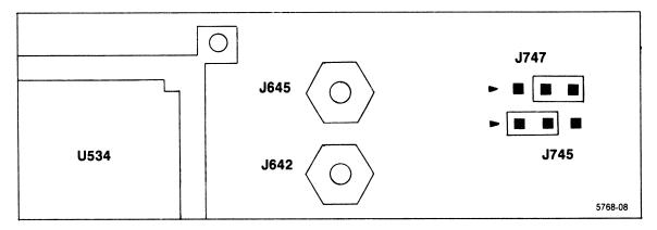
Figure B-8. Multiple 91HS8 position for jumper 745.
