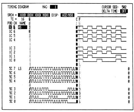
Figure 9. 91A32 ARMS 91HS8 Timing Diagram.
