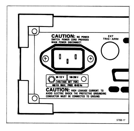
Figure B-1. 91HS8 cabinet voltage indicator screw.
