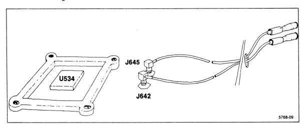
Figure B-9. Connecting clock cables to the 91HS8 Acquisition board.
