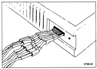
Figure 4. Connecting probes to front-panel calibrator pins.
