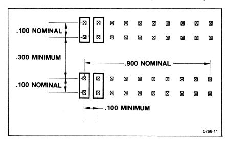
Figure 1. Minimal square pin spacing for 91HS8 probelets.
