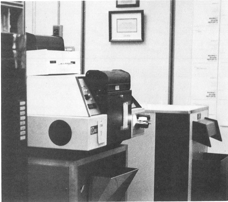
Fig. 4. Once translated by the Kennedy, the typesetting specifications and text data are sent to the Photon typesetting processor.
