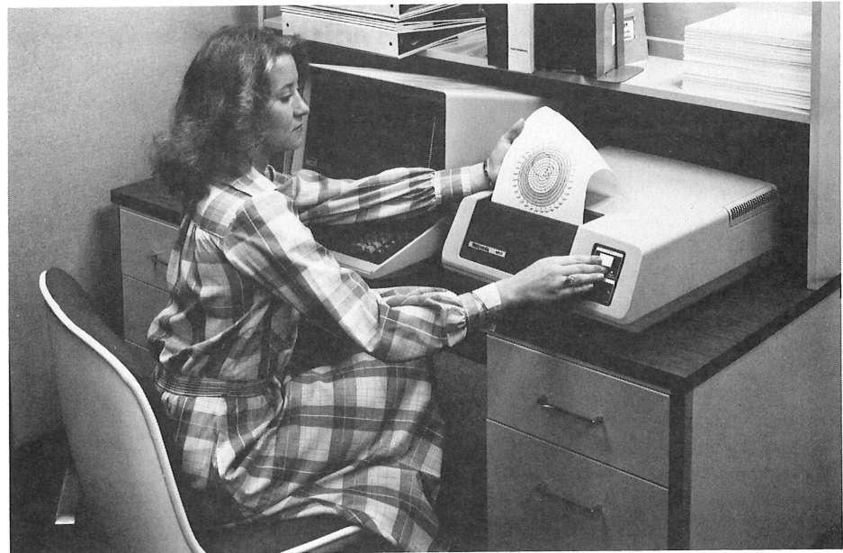
Fig. 1. The new 4611 Hard Copy Unit is based on an innovative new implementation of electrostatic technology.
