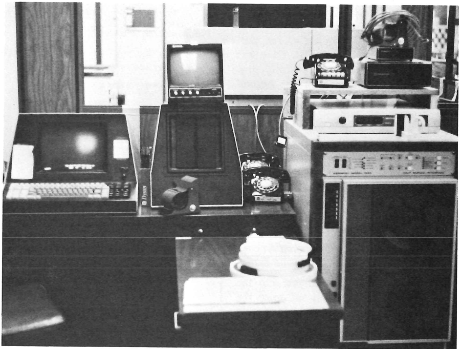
Fig. 3. The data from the 4051 is captured on the Alpha Key FDTs III terminal (left) and transferred to the Kennedy drive and tape (right).
