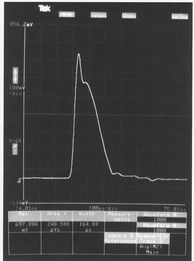
Figure 4. The OIG 502 high-energy optical impulse as captured by a Tektronix CSA 803 Communications Signal Analyzer with an SD-26 Sampling Head and SD-46 Optical to Electrical Converter.
