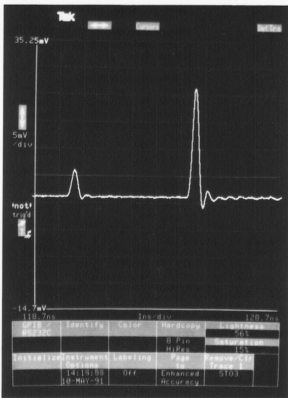
Figure 7. A set of typical optical reflection displays. The pulses displayed on the oscilloscope will be attenuated by losses introduced from two passes through the optical splitter
