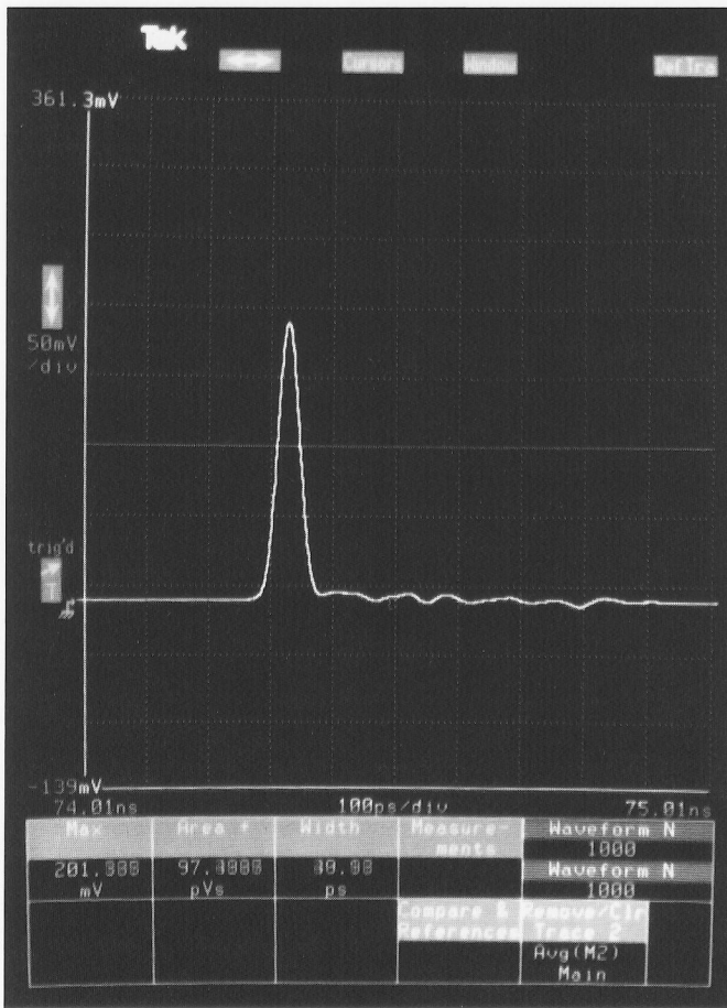
Figure 3. The OIG 502 low-energy impulse as captured by a Tektronix 11810A sampling oscilloscope with an SD-26 Sampling Head and SD-46 Optical to Electrical Converter.
