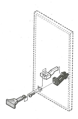
PLUG-IN LATCH ASSEMBLY DETAIL
