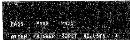
Figure 3. The EXT CAL menu showing that calibration routines for attenuator gain, trigger amplifier gain and offset, and repetitive mode ramps passed and parameters updated during the last time each routine was run.
