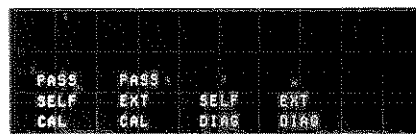
Figure 1. The CAL/DIAG menu showing PASS indications. These indicate that the SELF CAL and EXT CAL routines passed and parameters updated the last time they were run.
