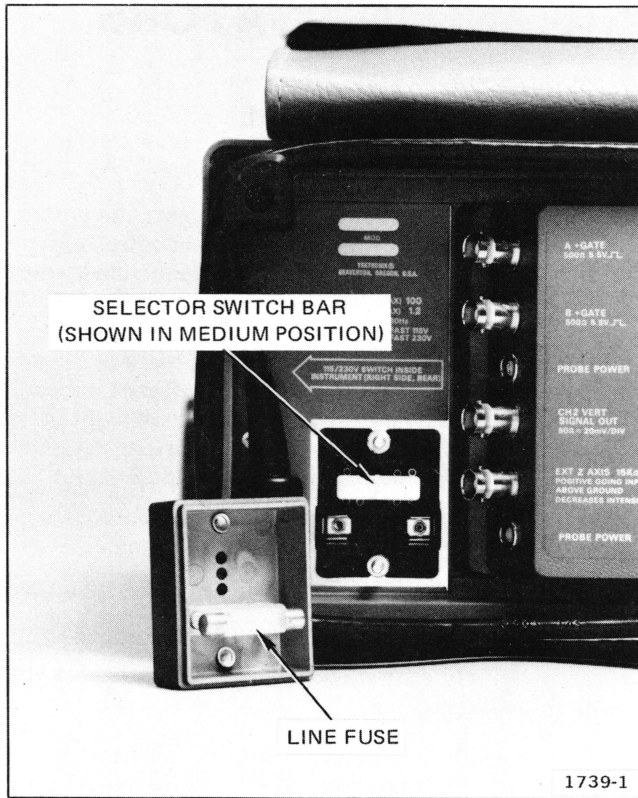
Fig. 1. Regulating range selector and line fuse.
