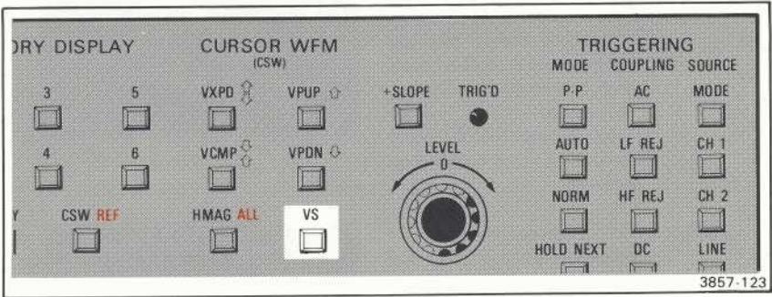
Figure 2-31. The VS (Versus) key.
