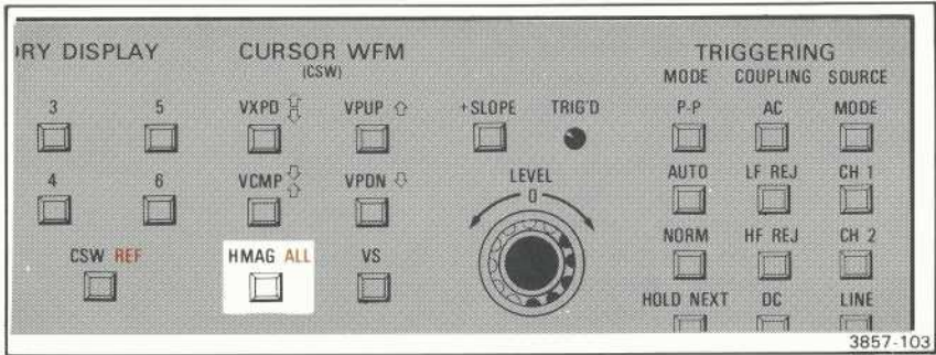
Figure 2-30. Horizontal Magnify ALL waveforms key.
