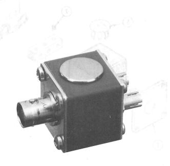
The 067-0562-00 P6046 Input Adapter is a device which connects the P6046 dual input tips together to the center conductor of a BNC connector. Mechanically, the electrical length of both inputs is made equal. This achieves high-frequency signal cancellation during the 50 MHz 1000:1 common mode rejection calibration adjustments.
