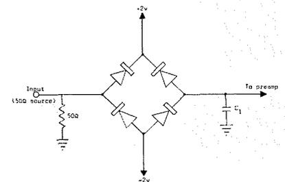
Figure 1. Schematic of a simplified sampling-bridge gate.
