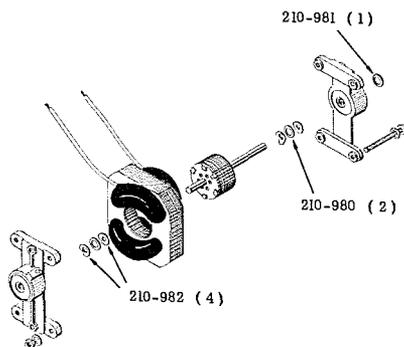
Figure 4. Exploded drawing of fan motor, part number 147-001.
