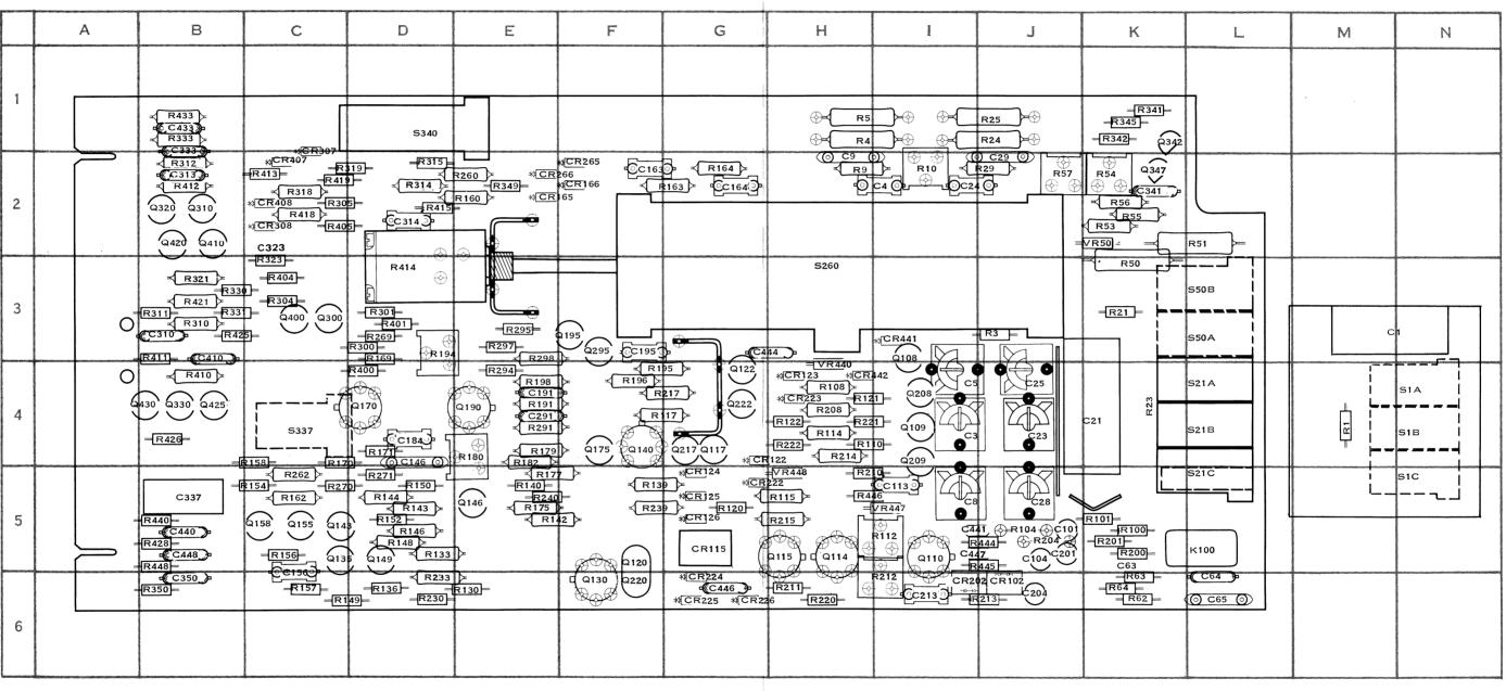
NOTE. COMPONENTS SHOWN WITH DASHED LINES ARE LOCATED ON BACK SIDE OF BOARD.
