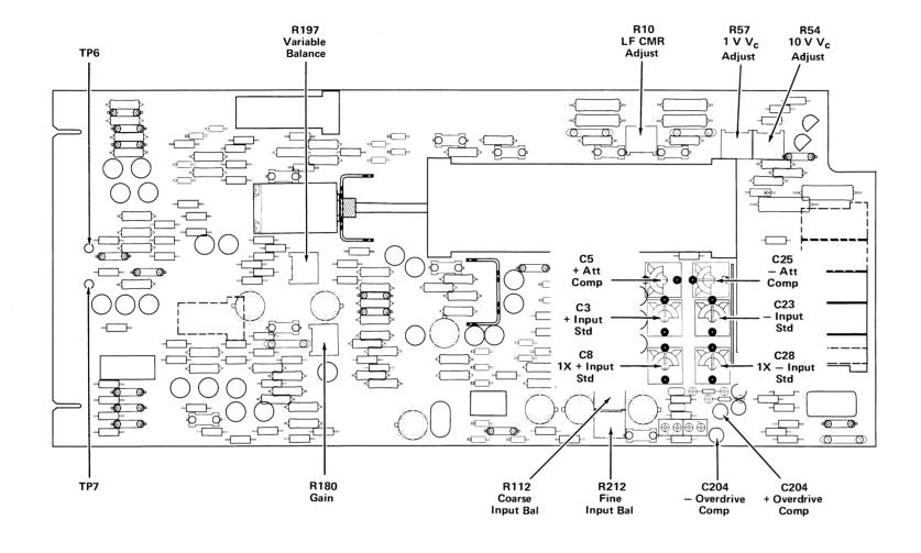
Fig. 4-2. Location of internal controls and test points.
