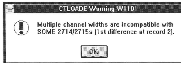
Figure C-30: The Message box warning that multiple channel widths are incompatible with some 2714 and 2715 instruments
