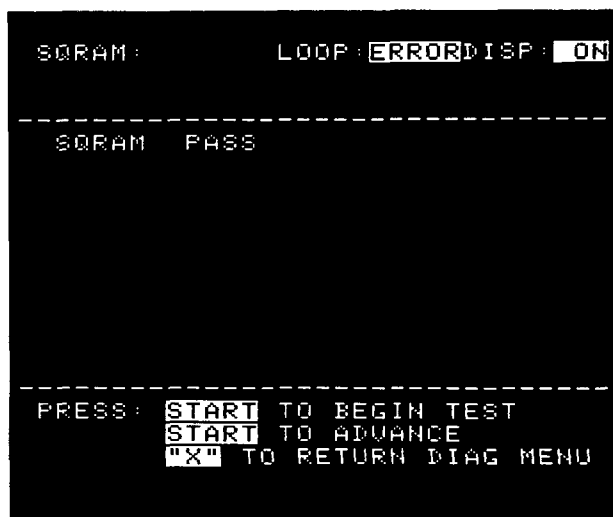
Figure 2-14. Display for trigger sequencer's RAM tests.
