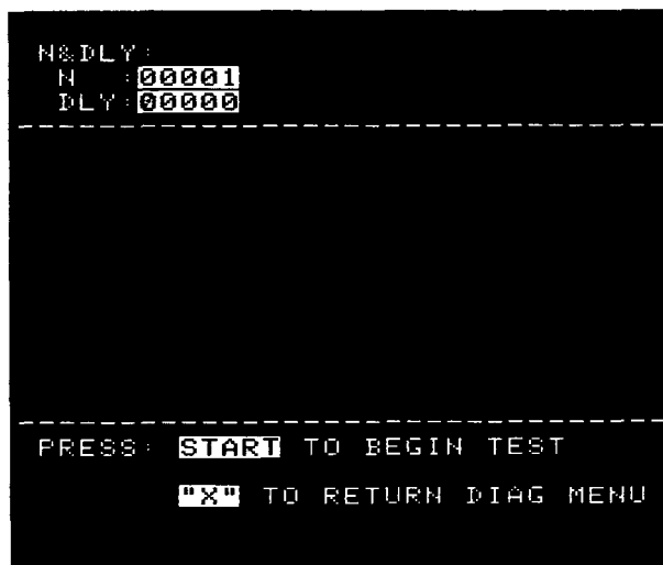
Figure 2-15. Display for N counter or DLY counter tests.
