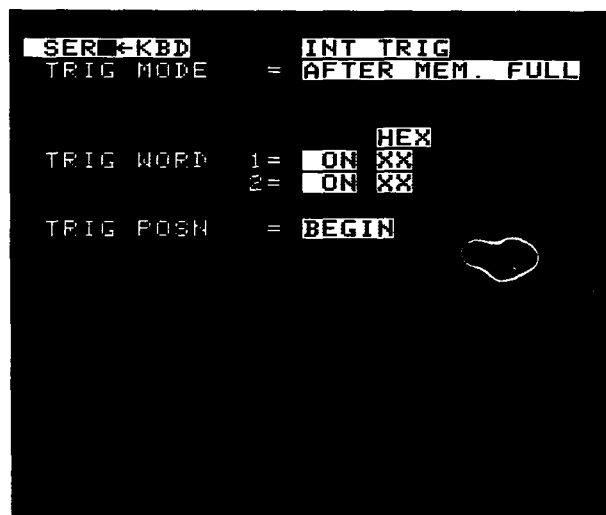
Figure 5-3. Default display of the Trigger menu.
