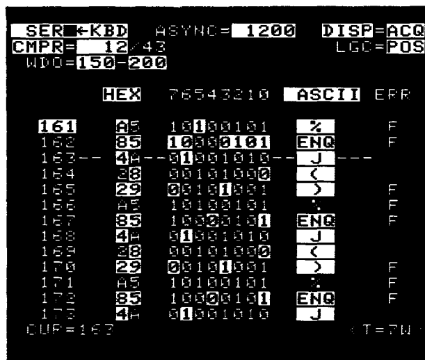
Figure 7-14. State Table CMPR display of serial acquisition.
