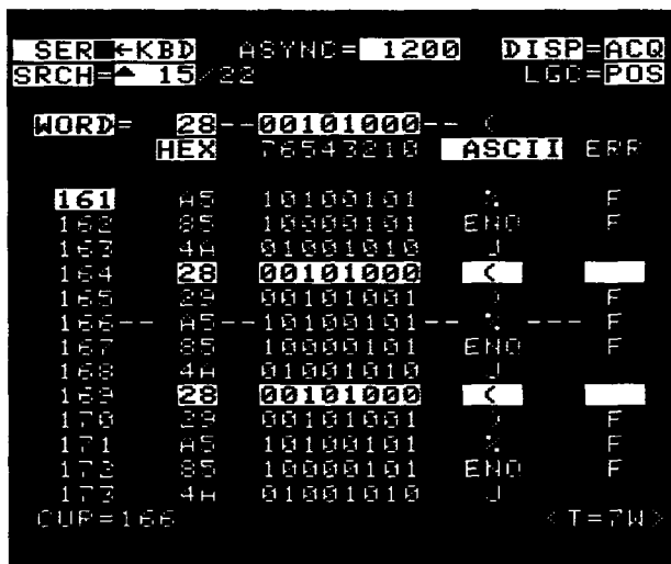
Figure 7-13. State Table SRCH display of serial acquisition.
