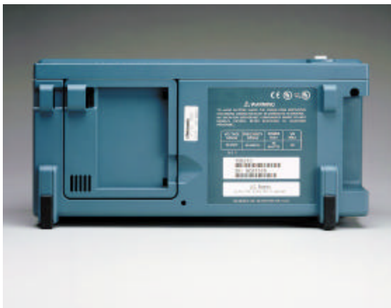
Rear panel view of a Tektronix TDS 210. The larger horizontal white label displays the model and serial numbers.
