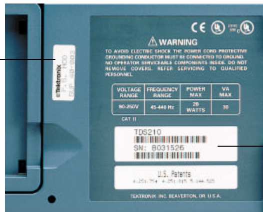
This vertically oriented white decal in about the center of the rear panel, marked "P.S. MOD SUP 40-003," indicates that the oscilloscope has been modified.
