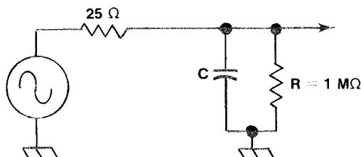
(B) Oscilloscope with high input impedance
