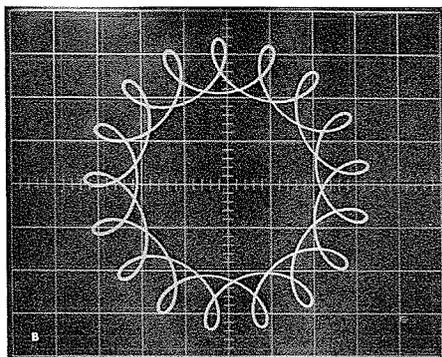
Fig. 2. Typical roulettes for a 15:2 frequency ratio.
