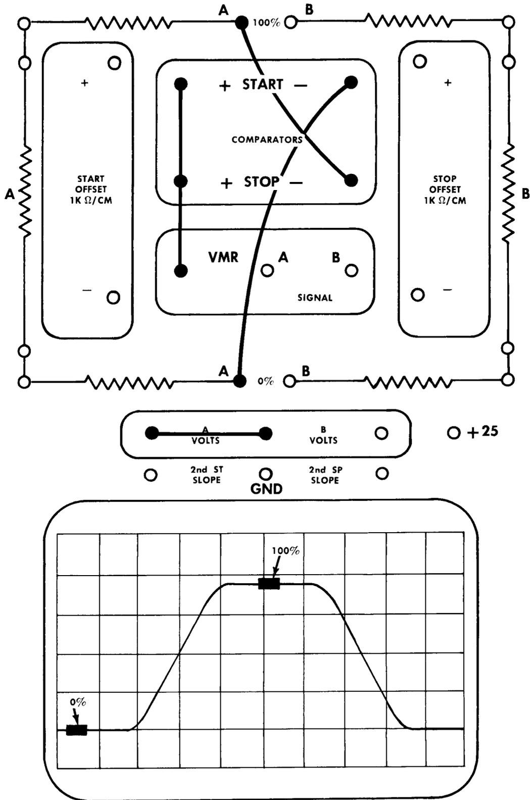
Fig. 3-1. Program card wired for a channel A voltage measurement.
