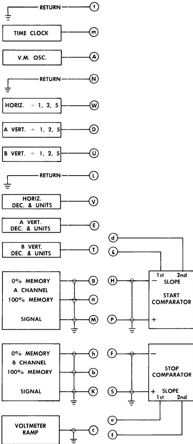
Fig. 4-2. Circuits used to interconnect an external program.
