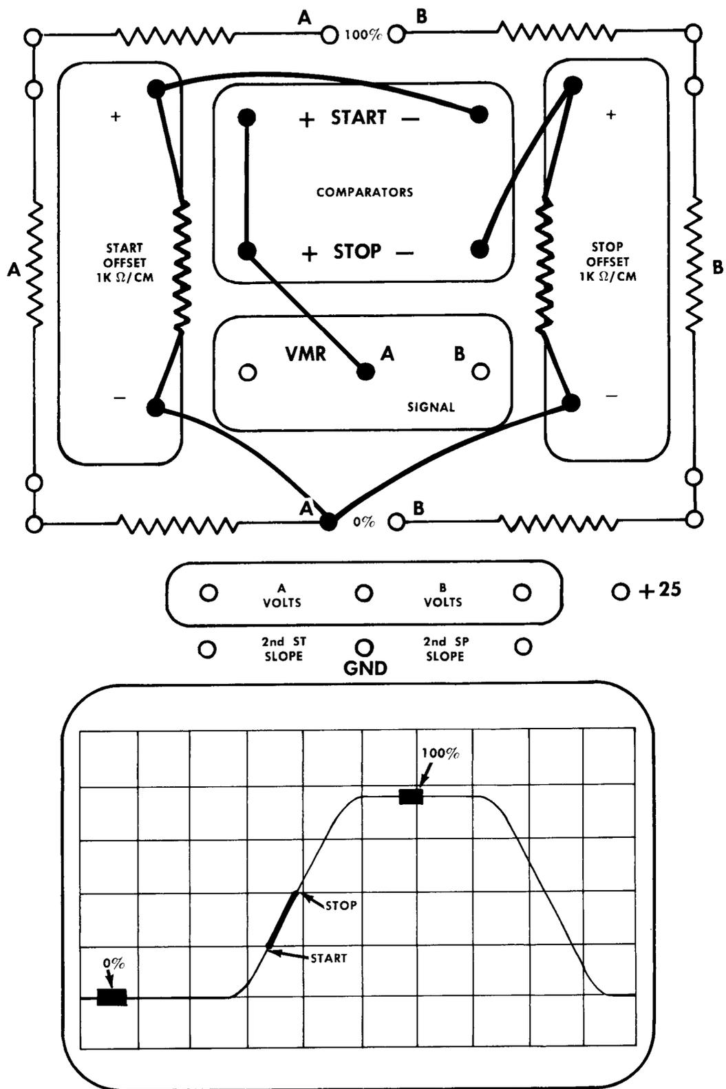
Fig. 3-8. Program card wired for an A signal rate-of-rise measurement with the Start-to-Stop Zone 1-cm up from the 0% and 2-cm up from the 100% zones.
