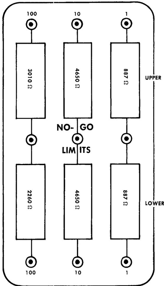
Fig. 3-10. Program card NO-GO LIMITS section wired for 350 upper limit and 250 lower limit.
