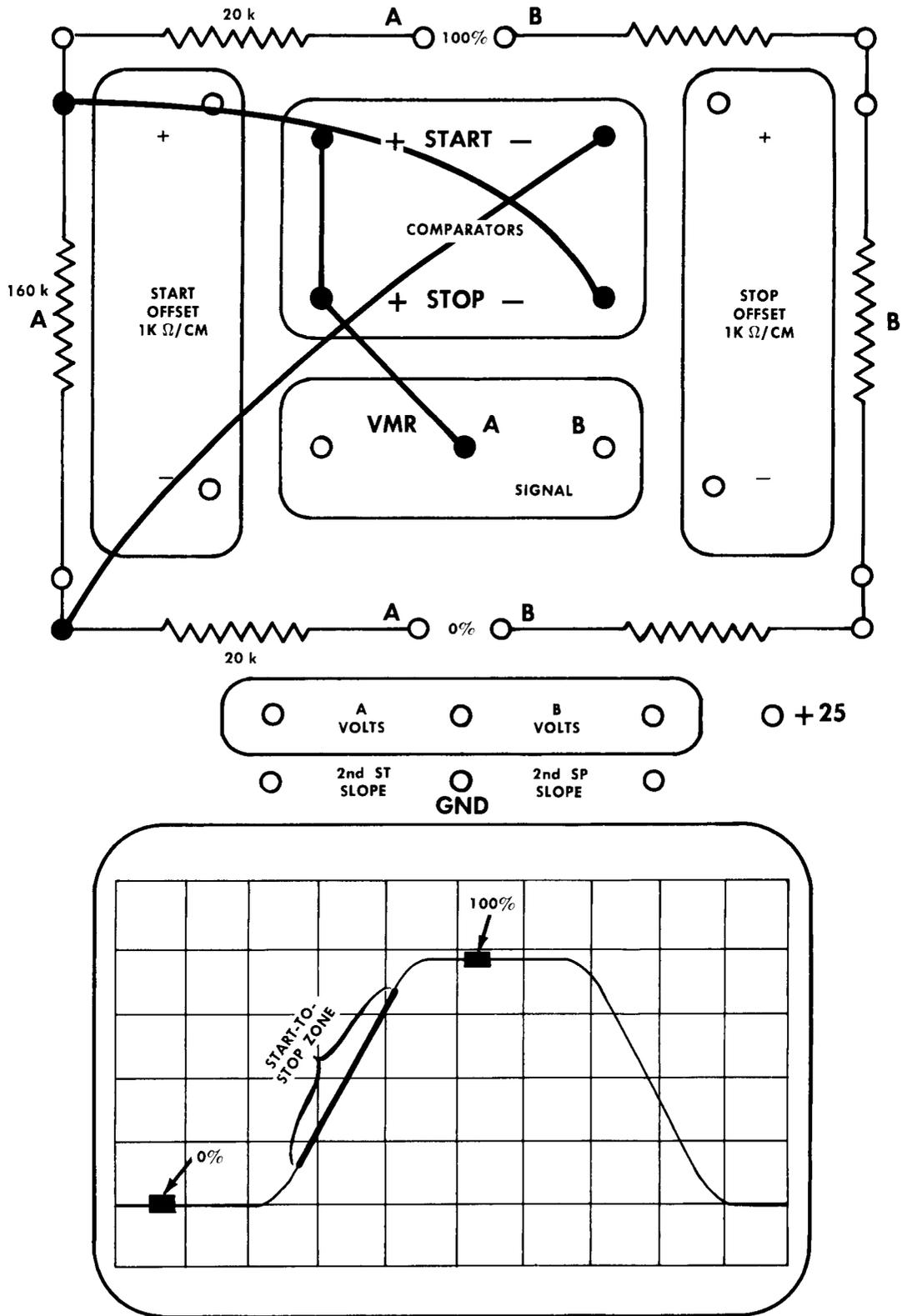
Fig. 3-3. Program card wired for an A signal risetime measurement with the Start-To-Stop Zones between the 10% and 90% zones.
