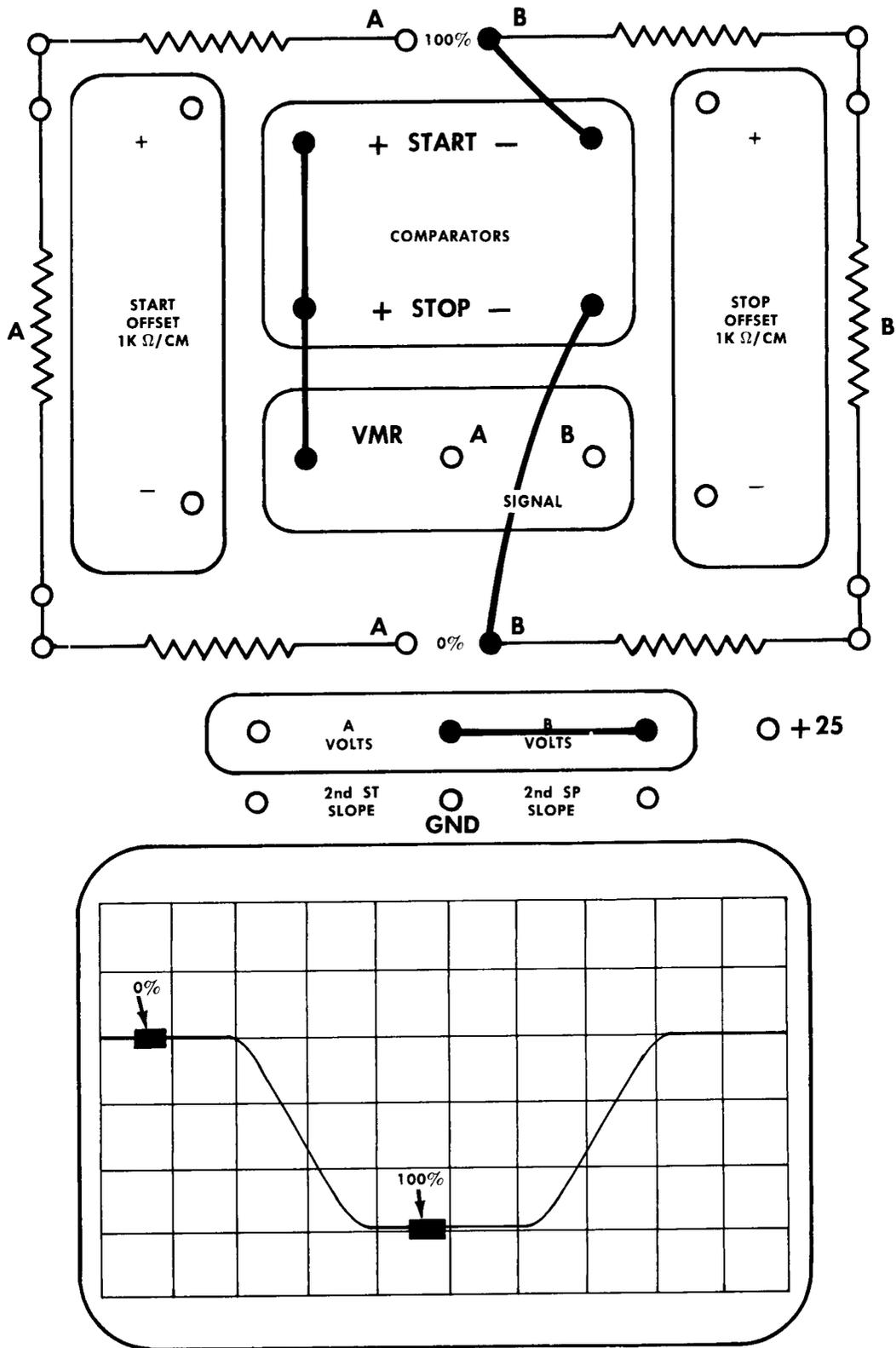
Fig. 3-2 Program card wired for a B voltage negative-going signal measurement between the 0% and 100% zones.
