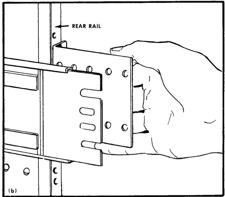
Fig. 2-4. Determining the mounting position of the slideout track stationary section on the cabinet rear rail: (a) normal position, inside the rear rail; (b) reverse position, outside the rear rail.
