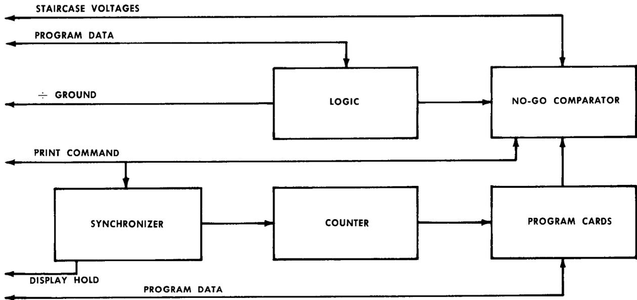
Fig. 4-3. Circuits used for automatic operation.
