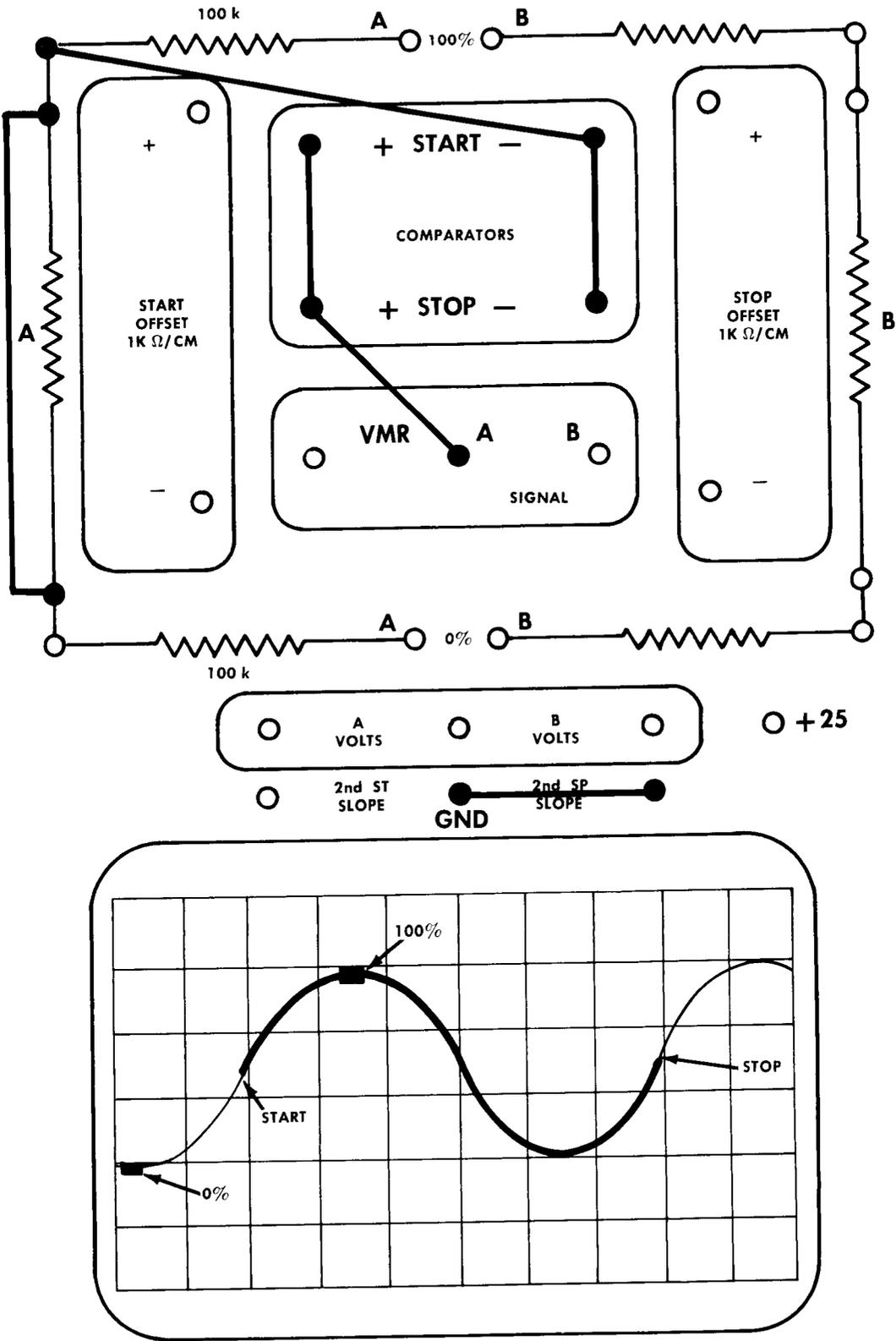
Fig. 3-9. Program card wired for an A signal period of 1 cycle measurement with the Start-To-Stop Zone between the A 50% 1st + Slope and the A 50% 2nd + Slope.
