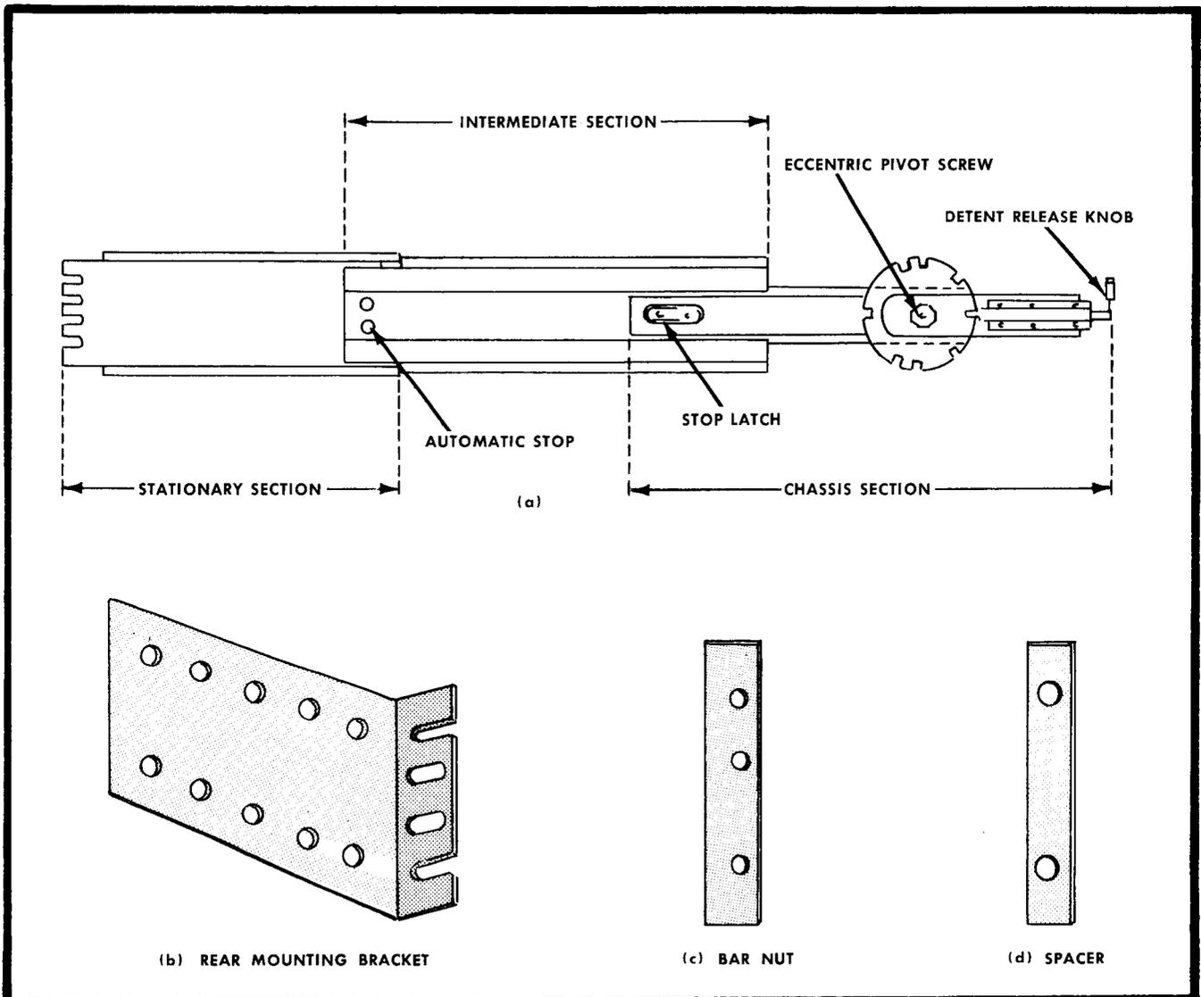
Fig. 2-1. Slideout track assembly.
