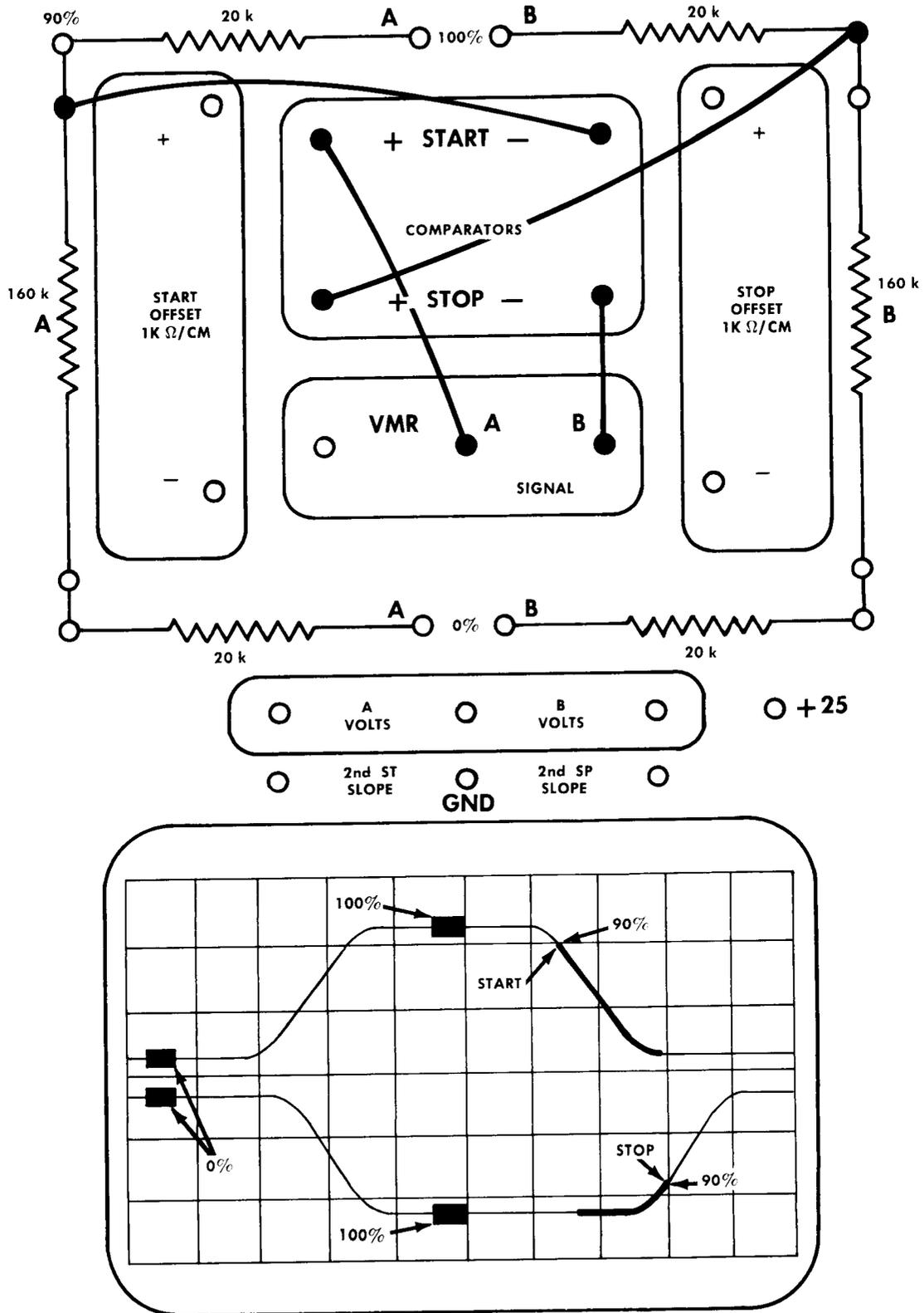
Fig. 3-7. Program card wired for an A signal to B signal storage measurement with the Start-To-Stop Zone between the A 90% 1st - Slope and the B 90% 1st + Slope.
