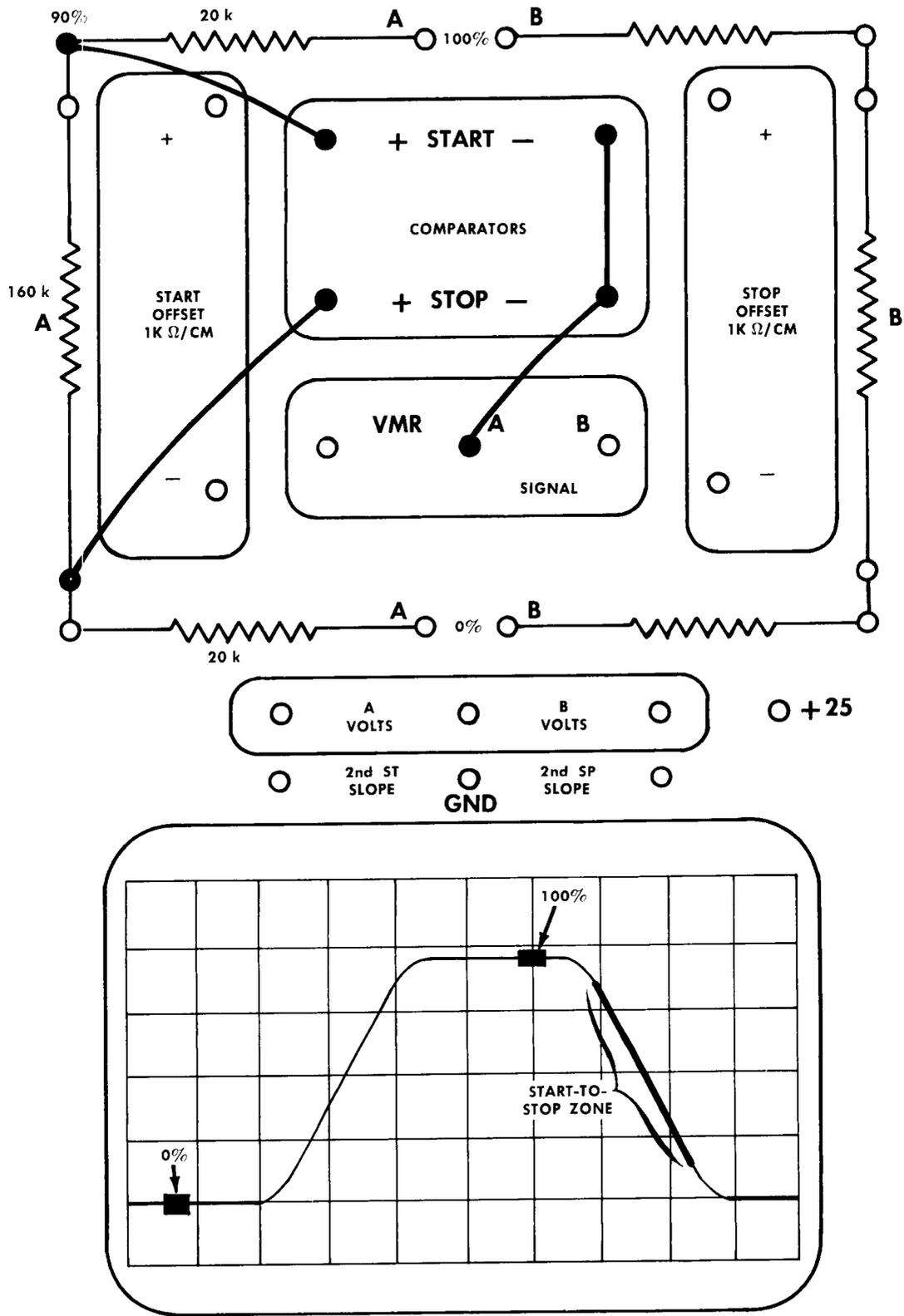
Fig. 3-4. Program card wired for an A signal falltime measurement with the Start-To-Stop Zone between the 90% and 10% zones.
