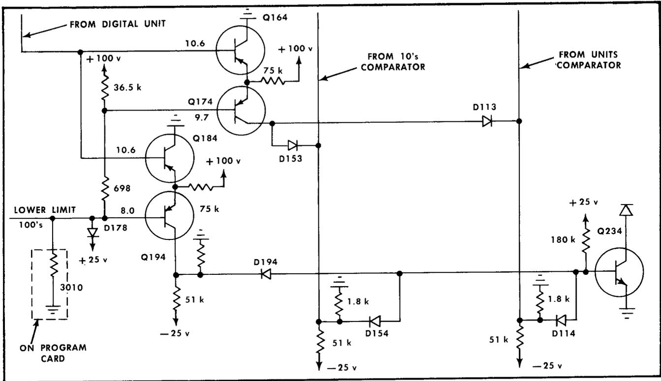
Fig. 4-4. Simplified schematic of the lockout comparator.
