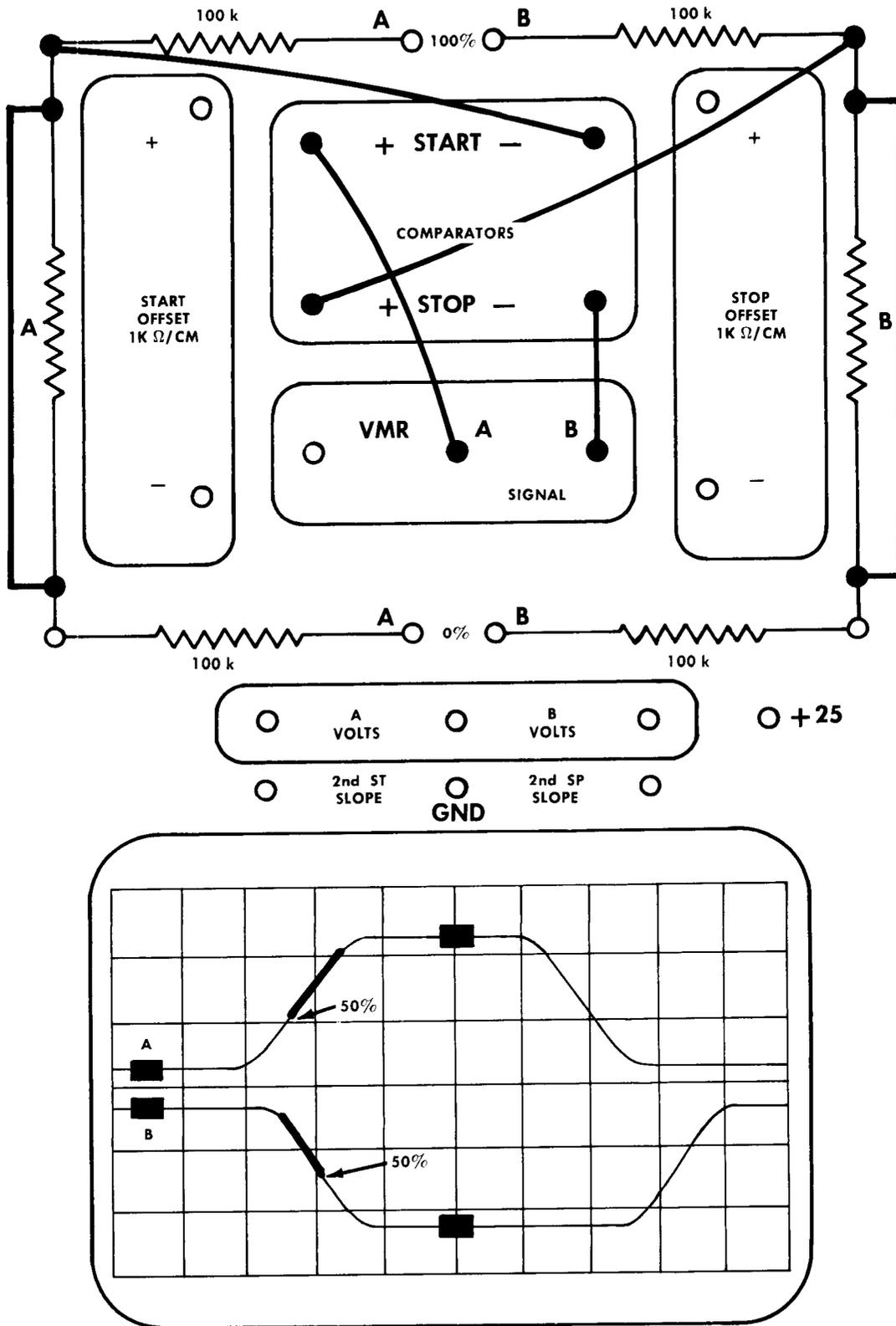
Fig. 3-6. Program card wired for an A signal to B signal delay measurement with the Start-To-Stop Zone between the A 50% 1st + Slope and the B 50% 1st - Slope.
