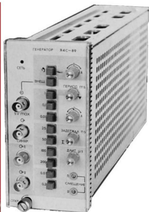
Differential generator block voltage Ya4S-89. 1978
