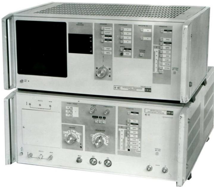
Special oscilloscope S9-6 with a bandwidth of 100 MHz. 1980
