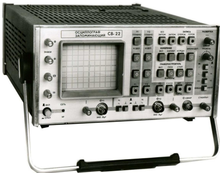
Combined oscilloscope C8-22. 1987
