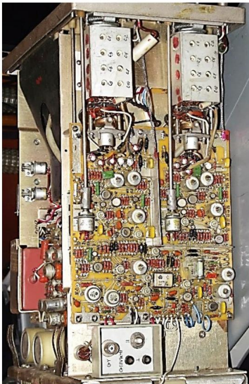
Oscilloscope S1-93 inside
