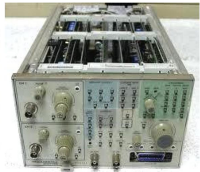
Tek 7D20 sampler unit
