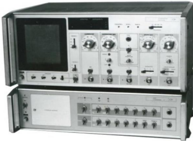
Digital oscilloscope S9-10/1. 1982
