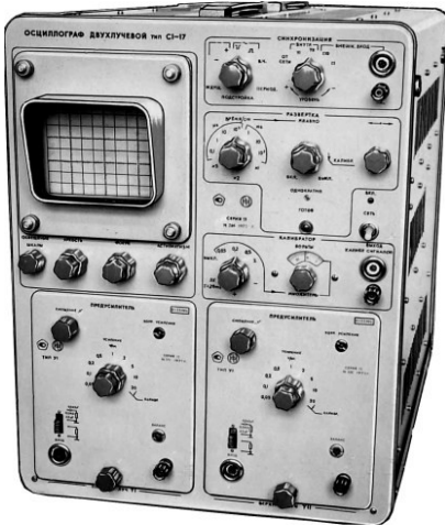
Two-beam oscilloscope with interchangeable units C1-17 "Bahroma-B", 1961.
