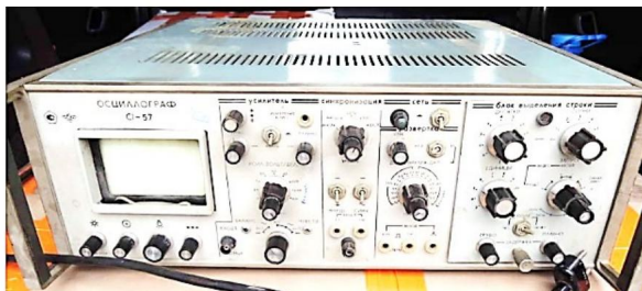
Special television oscilloscope S1-57 (S9-57)
