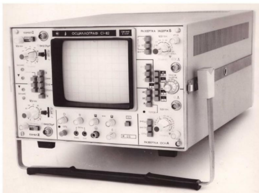
2-channel oscilloscope S1-82 (10 MHz)
