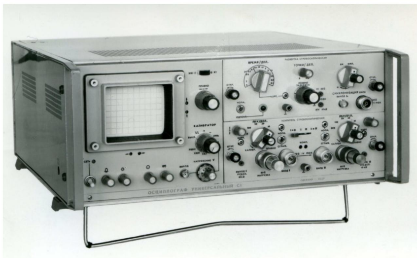
Stroboscopic version of the universal oscilloscope S1-70 with replaceable stroboscopic units 1U71 and 1R71. 1972
