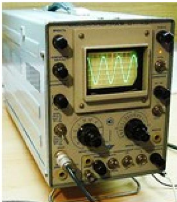
Small-sized semiconductor oscilloscope S1-49
