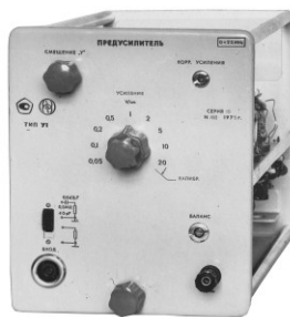
Single channel preamplifier U1
