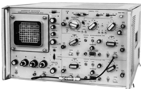
Dual beam storage oscilloscope with replaceable blocks C8-14. 1974
