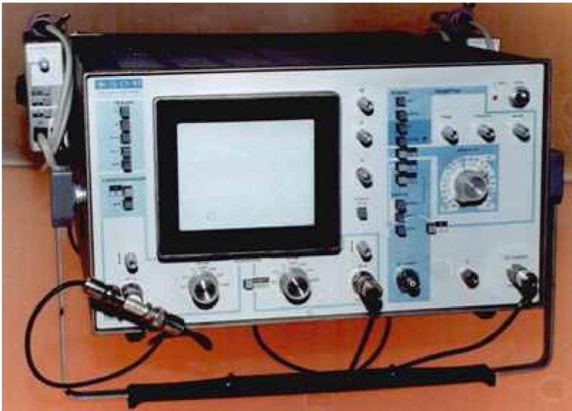
Universal two-channel oscilloscope C1-97. 1979 The active probe is visible on the left.
