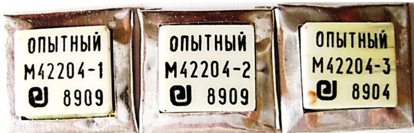
Broadband amplifier chips for a band up to 2-4 GHz
