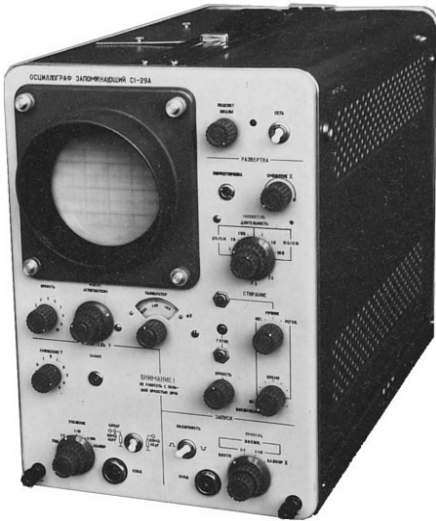
1- The C8-9 (C1-29) storage oscilloscope. 1964 г.
