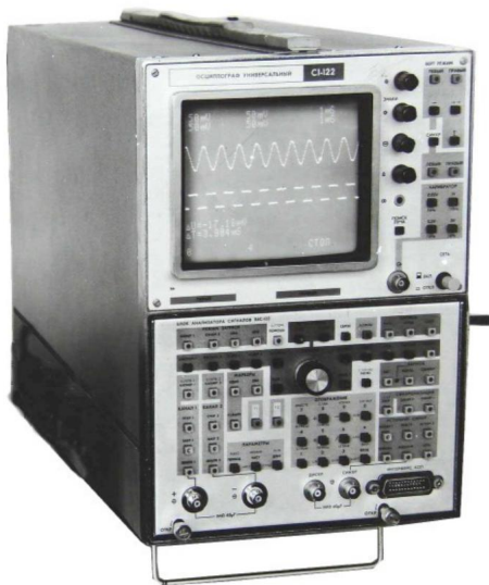
Universal digital oscilloscope S1-122/8 (with signal analyzer unit YA4S-122) 1986
