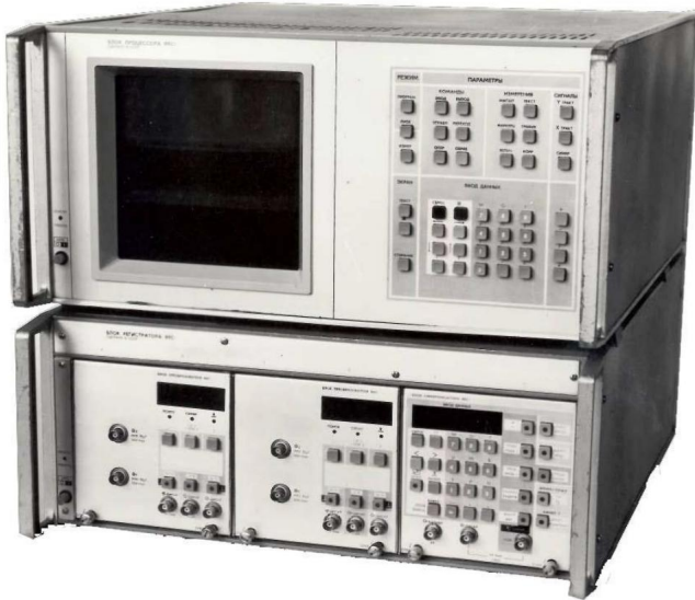
Computational oscilloscope S9-20 with a maximum sampling frequency of 100 MHz. The oscilloscopes S9-21, S9-22 and S9-23 were developed in a similar configuration. 1986
