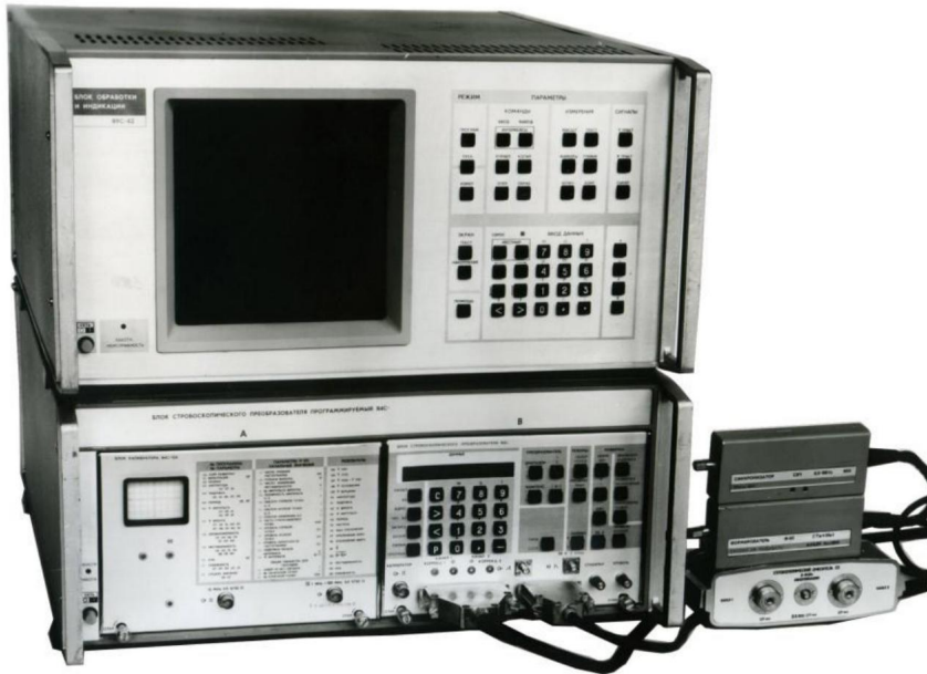
Stroboscopic oscilloscope C7-20/4 at 30 GHz, 1990
