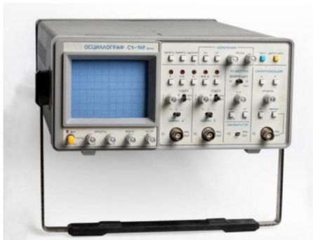
2-channel, midrange, analog-digital oscilloscope S1-149 (50 MHz) .
