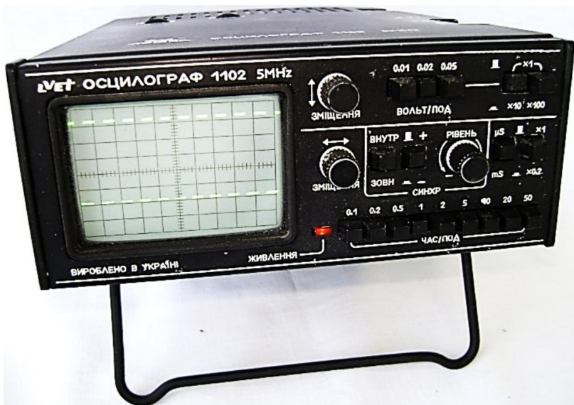
Oscilloscope 1102 (A) for 5 (20) MHz band
