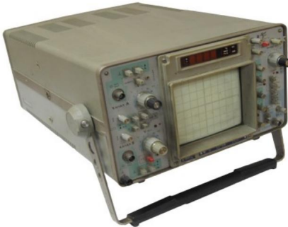
2-channel oscilloscope S1-114 with a multimeter at 50 MHz.
