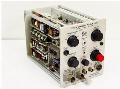
Replacement strobe unit Tek "N", per lane 500 MHz. 1960 r.
