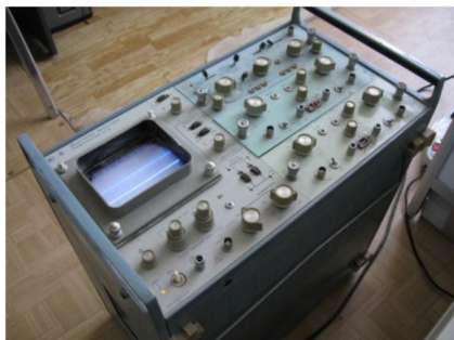
Dual-beam oscilloscope with replaceable blocks S1-74. 1974
