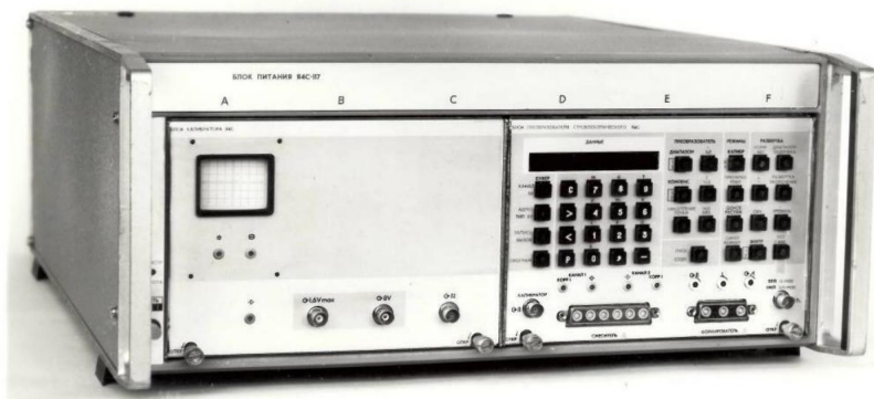
Precision stroboscopic transducer YA4S-125, consisting of a base unit YA4S-117, in which the calibrator unit YA4S-124 (left) and the stroboscopic transducer unit YA4S-123 (right) were located. The Sheaf-Blueberry version came with a 10 GHz mixer. 1986
