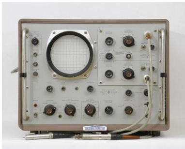
HP 185A stroboscopic oscilloscope, for the 500 MHz band. 1960 r.
