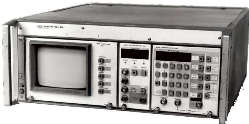
Digital oscilloscope S9-26 with a four-channel multiplexer unit YA4S-116. In a similar configuration oscilloscopes S9-24 and S9-25 were developed. 1986
