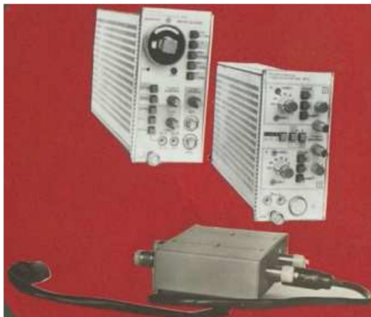
Replaceable stroboscopic blocks YA4S-96, YA4S-95 and stroboscopic mixer. 1978
