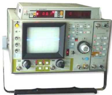
SP Oscilloscope C1-116 at 250 MHz.
