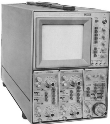
Universal oscilloscope with replaceable blocks S1-91. 1977
