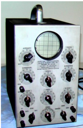
DuMont 164 Oscilloscope (30 kHz band) 1940.
