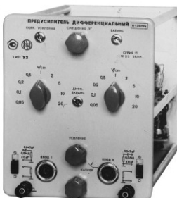
Differential preamplifier U2
