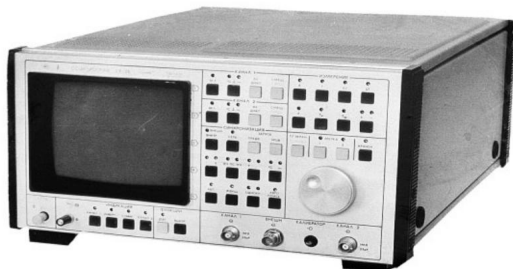
ShP digital oscilloscope S9-28 at 100 MHz - weight 12 kg.
