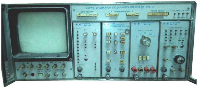
Oscilloscope SK1-95 at 100 MHz , with amplifier Ya4S-80, scanner Ya4S-83, multimeter Ya4S-87 and measurements Ya4S-84.
