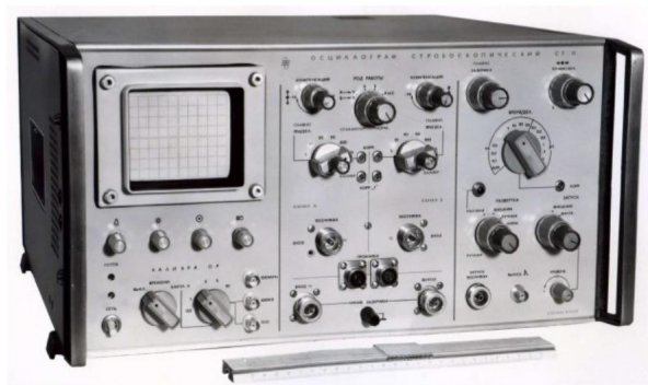
Stroboscopic oscilloscope S7-11. 1971
