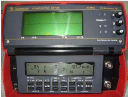
Digital service oscilloscope S8-28 , 20 MHz, weight 3 kg.
