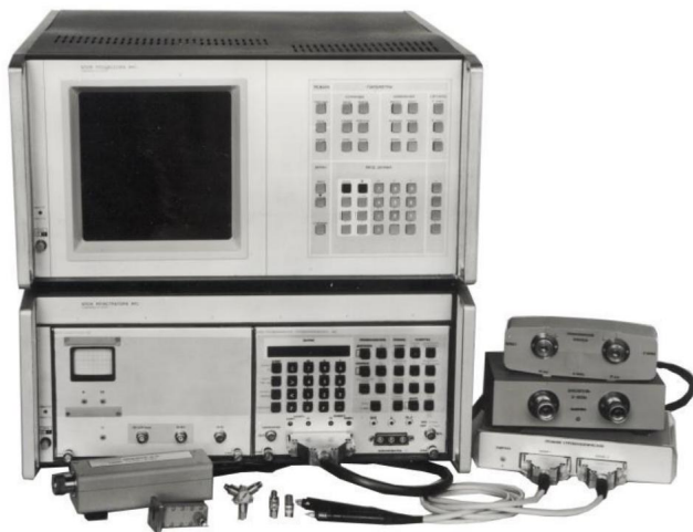
Computational stroboscopic oscilloscope C7-20 with replaceable mixers and voltage difference generators. 1987
