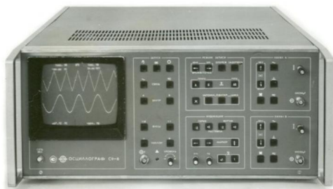
2-channel digital oscilloscope S9-8 (2.5 MHz, 20 MV/s)
