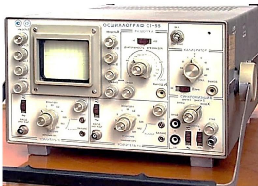
Dual-beam oscilloscope S1-55
