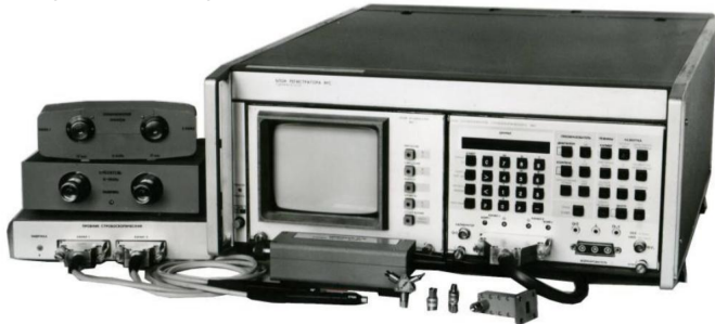
Stroboscopic oscilloscope C7-21 with replaceable mixers and voltage differential generators. 1988
