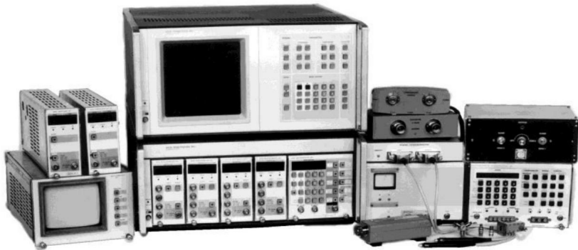
Devices and units included in the family of digital and stroboscopic oscilloscopes "Sputnitsa" / "Sheaf" / "Sofia"
