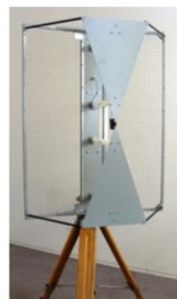
Loaded Bow-Tie Antenna GZ00803ANL 0.08 ÷ 0.3 GHz
