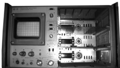
Photo of the base unit of the S1-74 oscilloscope without inserted replaceable units
