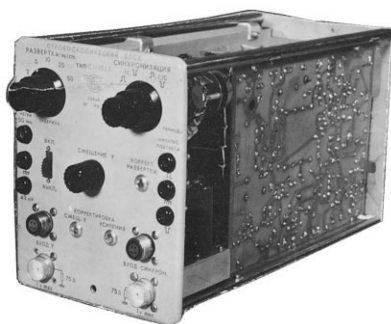
Replaceable strobe unit U7 with bandwidth 200 MHz, for C1-15/17. 1965 г.
