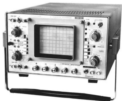
Storage oscilloscope S8-15. 1976
