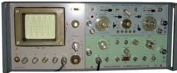
Legendary universal oscilloscope C1-70 with interchangeable units with 1U11 amplifier and 1P11 scanning units. 1972
