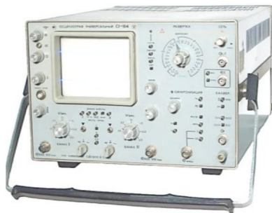
Universal WB oscilloscope C1-104 at 500 MHz. 1981
