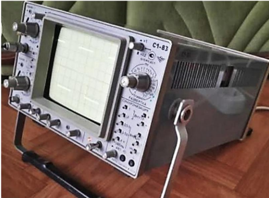
2 channel LF oscilloscope S1-83
