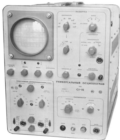
1st oscilloscope with interchangeable blocks in the country C1-15 ("Coolisa").1961.
