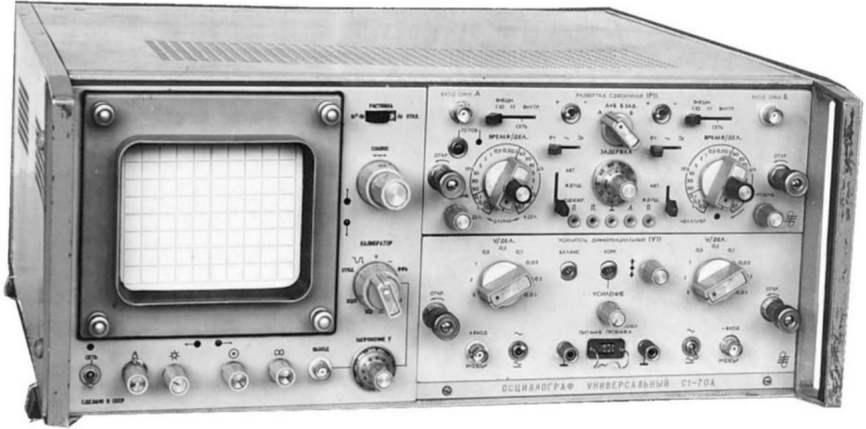
Universal oscilloscope C1-70A on a CRT with screen dimensions 80x100 mm. 1974
