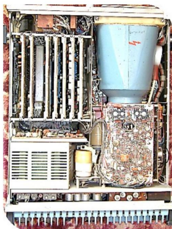
Automated oscilloscope S1-98 from the inside
