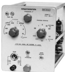
Highly sensitive differential amplifier U5
