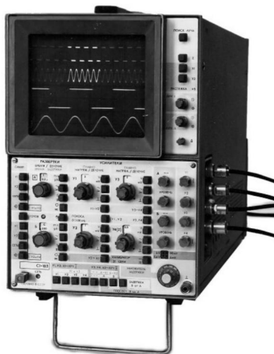
Dual beam four channel oscilloscope C1-103. 1979
