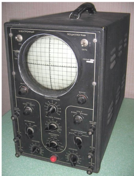
The first domestic oscilloscope S1-1 (EO-7). 1948 г.
