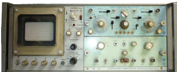
Storage oscilloscope with replaceable blocks C8-12. 1974
