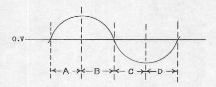
29. Given the signal shown at the lower right, what sweep range setting would you use to observe a maximum of 3 complete cycles on the face of a CRT which has 10 cm of vertical deflection and 10 cm of horizontal deflection:
