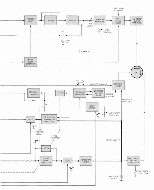
Fig. 2-6. Random-mode block diagram.
