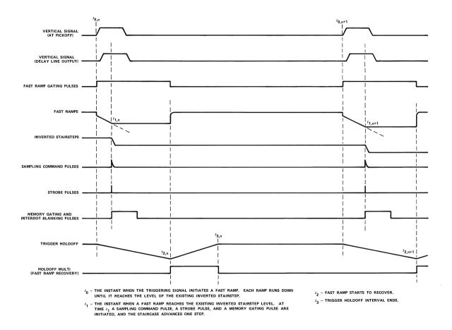
Fig. 2-4. Sequential-mode timing diagram.
