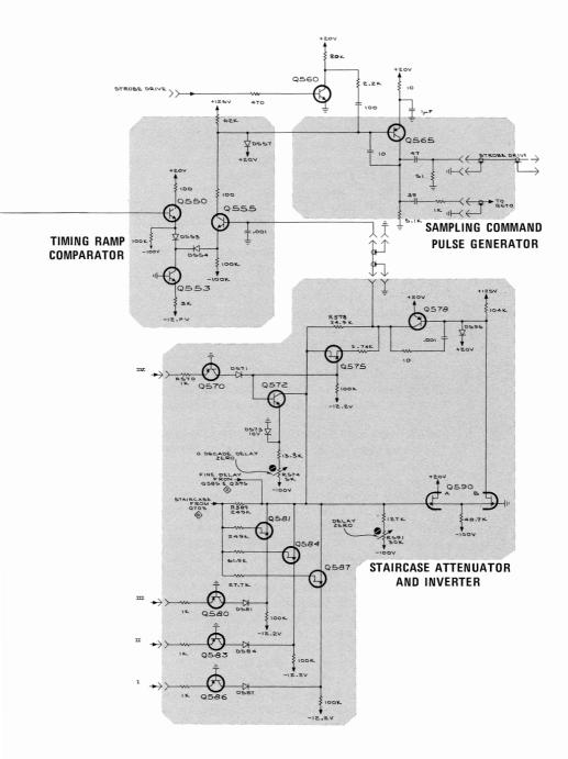
Fig. 5-5. 3T5 Timing Ramp and Staircase Inverter Amp.
