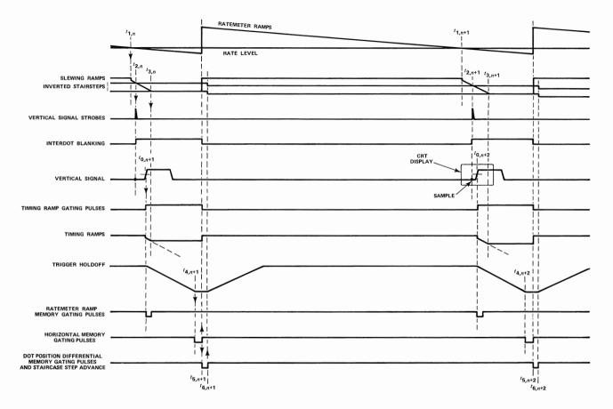
Fig. 2-7. Random-mode timing diagram.
