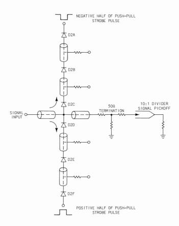
Fig. 3-13. Sampling-gate input.
