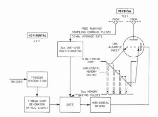
Fig. 2-10. 7T11 real-time mode (simplified).
