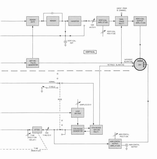
Fig. 2-3. Sequential-mode block diagram.
