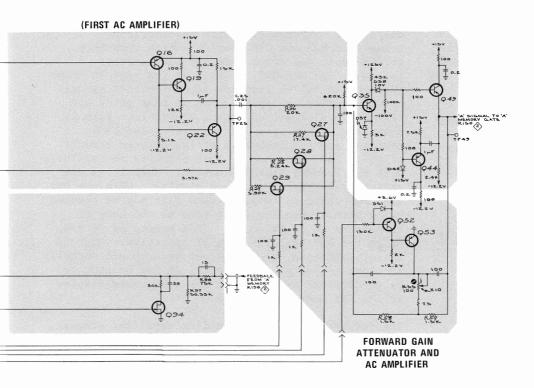
Fig. 3-6. 3S5 Ch A Programmed Amp and Attenuators.
