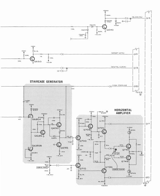
Fig. 5-7. 3T5 Staircase Gen and Horiz Amp.
