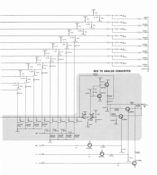
Fig. 5-6. 3T5 Delay Gating and Digital to Analog Converter.
