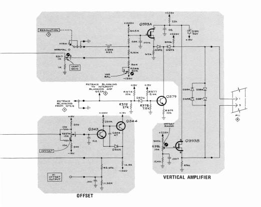
Fig. 3-3. 1S2 Offset and Output Stage.
