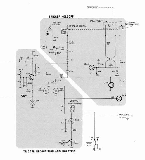
Fig. 4-8. 3T77A Trigger and Holdoff.
