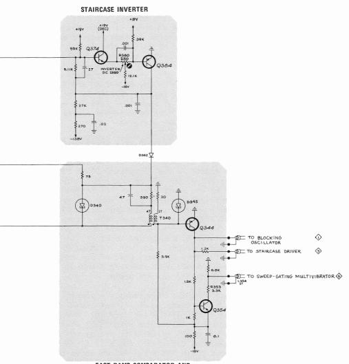
FAST RAMP COMPARATOR AND SAMPLING COMMAND PULSE GENERATOR
