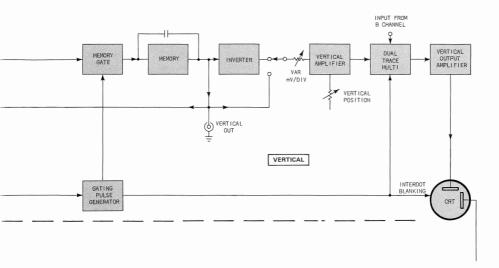
Fig. 2-1. Basic block diagram of vertical deflection section.
