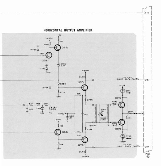
Fig. 6-3. 3T2 Horiz Amplifier and Blanking.
