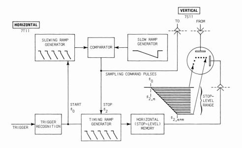
Fig. 2-5. 7T11 sequential mode (simplified).
