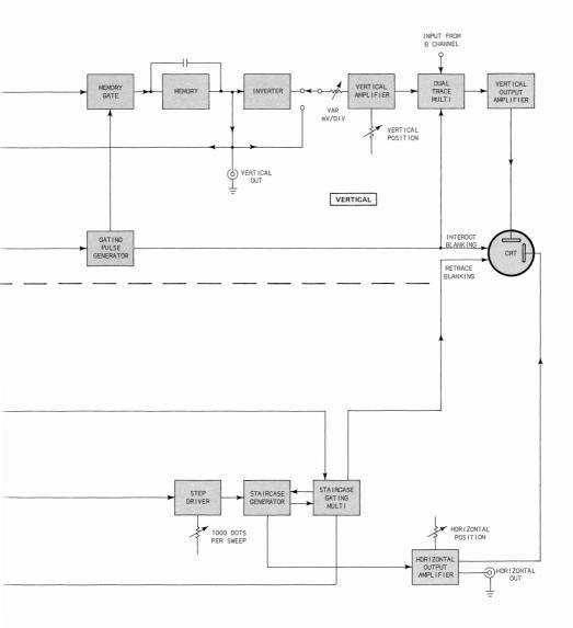
Fig. 2-9. Clocked real-time mode block diagram.
