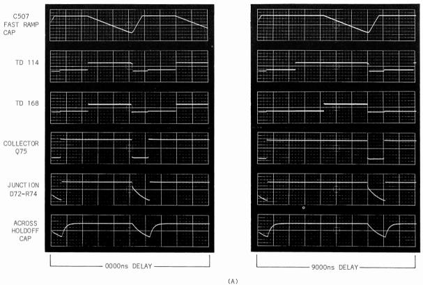
Fig. 4-7. Inside the 3T5. All oscillograms at 5 s/div (549-1A1).
