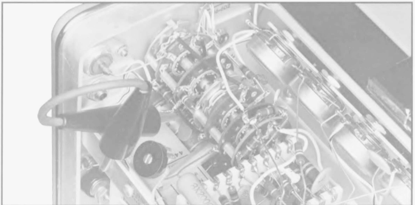
Fig. 5-3. Grounding the junction of R426, R427, R428 and C425.
