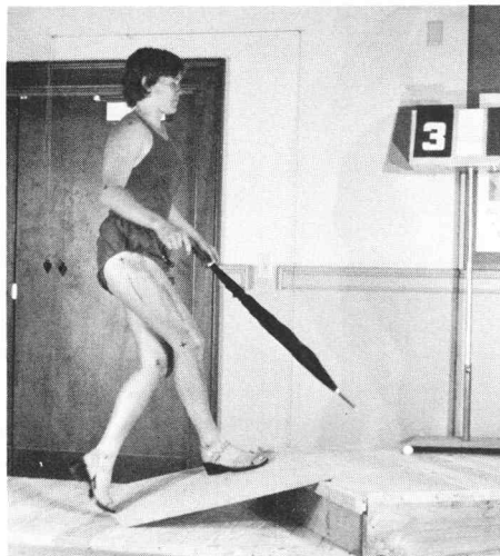
Fig. 8. A test subject attempting to negotiate the lab's ramp duplicate. The marks show key points to be digitized from film of the attempt.
