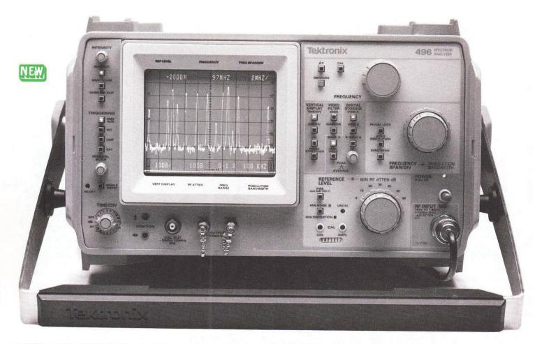
The 496P complies with IEEE Standard 488-1978. and with Tektronix Codes and Formats Standard
