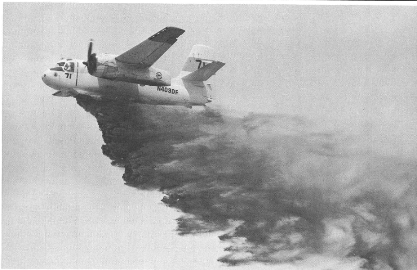
Aerial drops of fire retardants are analyzed at the Northern Forest Fire Laboratory in Missoula. How high and how much are two of the questions answered with the aid of a 4051.
