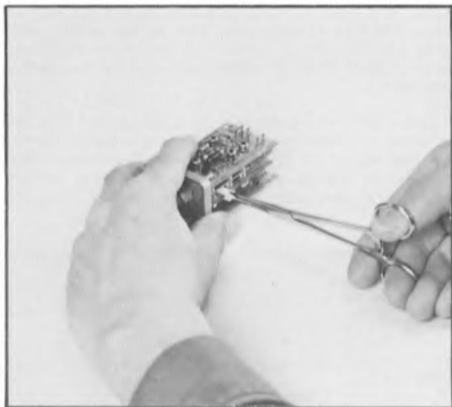
Fig. 4-2. Removal or replacement of sampling bridge diodes.
