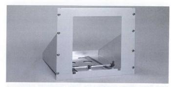
For rackmounting 500 and 7700-Series cabinet-type oscilloscopes in a standard 19-inch wide rack. Cradle mount consists of a cradle (or "shelf") without slide-out assemblies and a mask to fit over the regular instrument panel. 500-Series mask finish is blue vinyl, and 7700-Series mask finish is light gray.
