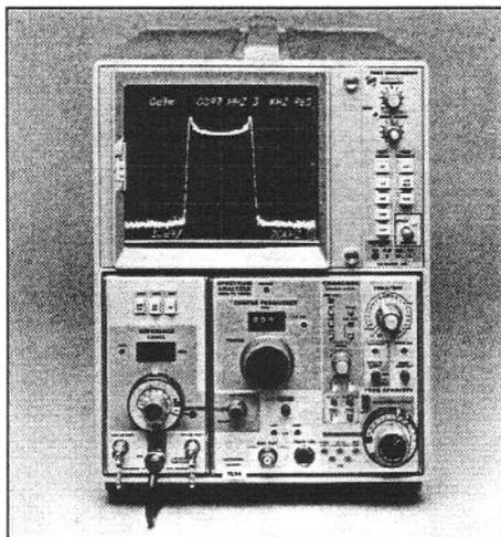
The 7L14 converts the 7603 Oscilloscope to a 1.8-GHz Spectrum Analyzer.
