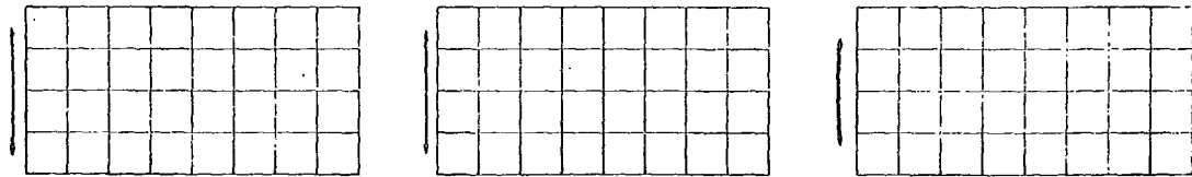
Fig. 16. Typical displays obtained with different settings of the GEOM ADJ control. The GEOM ADJ control should be set to obtain the display shown in the center illustration.
