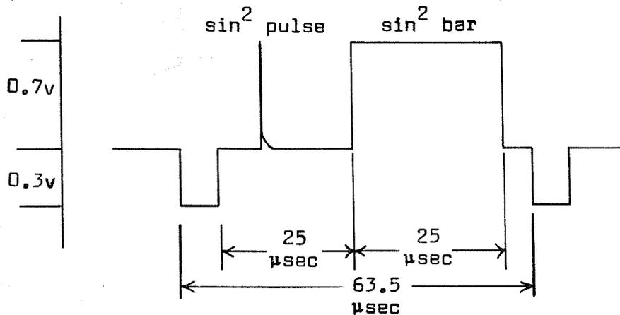
Figure 5. Composite test signal with typical time spacings.
