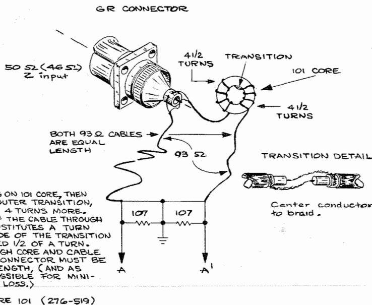
**Figure 3. Connector detail for direct connection to crt vertical plates — Type 580 Series Oscilloscope.**
