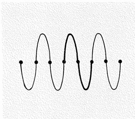
Figure 1. Sine wave with a single cycle indicated by the heavier line.
